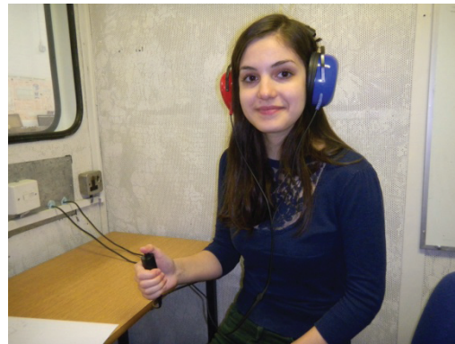
Figure 1: Audiometric booth showing response button and Audiocup TH49 headphones Copyright Stephen Dance 2014.
