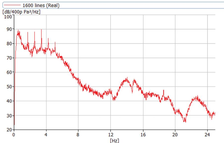
Figure 3: 1600 lines, 0 – 25 Hz FFT analysis – figure 55 from ref 4
