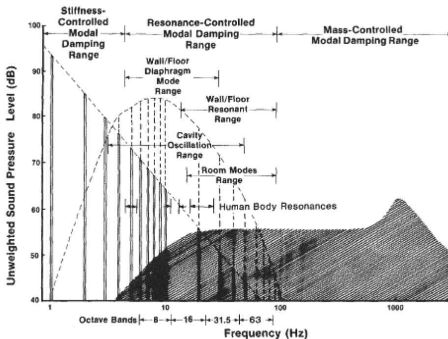
FIGURE 1: Turbine noise emission components with building and human body resonances superimposed. Ref [2]
