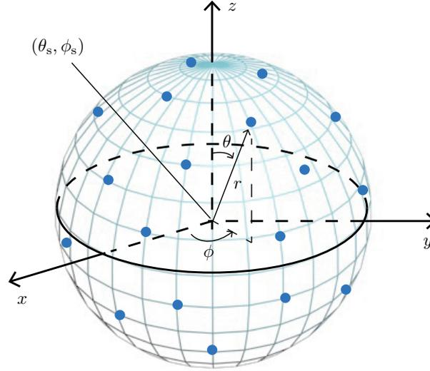
Figure 1. Illustration of a spherical microphone array in the Cartesian coordinate system, where  $(\theta_s, \phi_s)$  denotes the source incidence direction.
