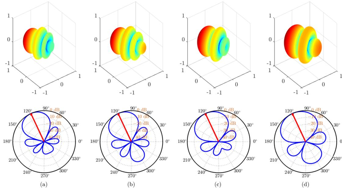
Figure 2. Beam patterns of the MAD beamformer with different values of  $\mathcal{W}_0$ : (a)  $\mathcal{W}_0 = -40$  dB, (b)  $\mathcal{W}_0 = -30$  dB, (c)  $\mathcal{W}_0 = -20$  dB, and (d)  $\mathcal{W}_0 = -10$  dB. Conditions of simulations:  $M = 32$ ,  $r = 3$  cm,  $f = 1$  kHz, and  $(\theta_s, \phi_s) = (90^\circ, 115^\circ)$ .
