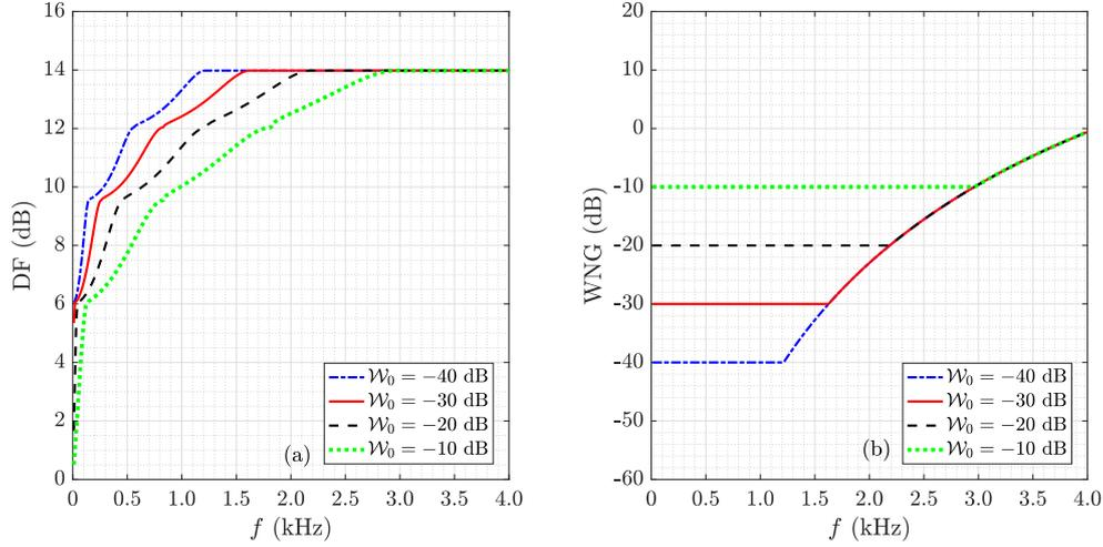
Figure 3. DFs and WNGs of the MAD beamformer as a function of the frequency,  $f$ : (a) DF and (b) WNG. Conditions of simulation:  $M = 32$  and  $r = 3$  cm.
