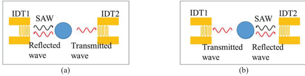
Figure 12 –Schematic illustration of droplet position detection. (a) SAW is generated from IDT1 and reflected and transmitted signals are measured by IDT2. (b) Vice versa.
