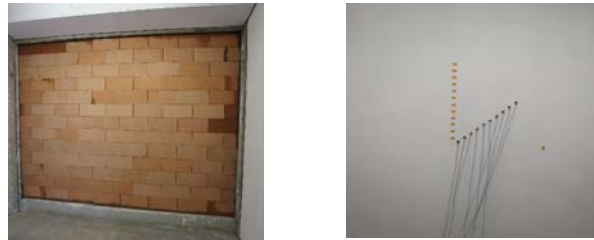
Figure 14 – Picture of the brick wall and the diagonal line of accelerometers
