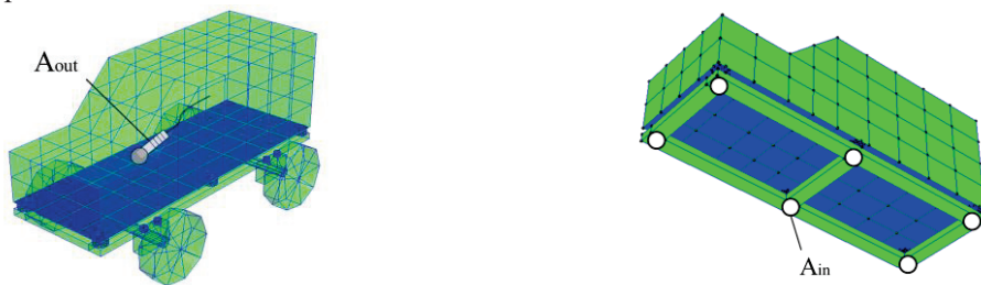
(a) OTPA PC model between body and interior noise (b) OTPA Ref model between frame and body
