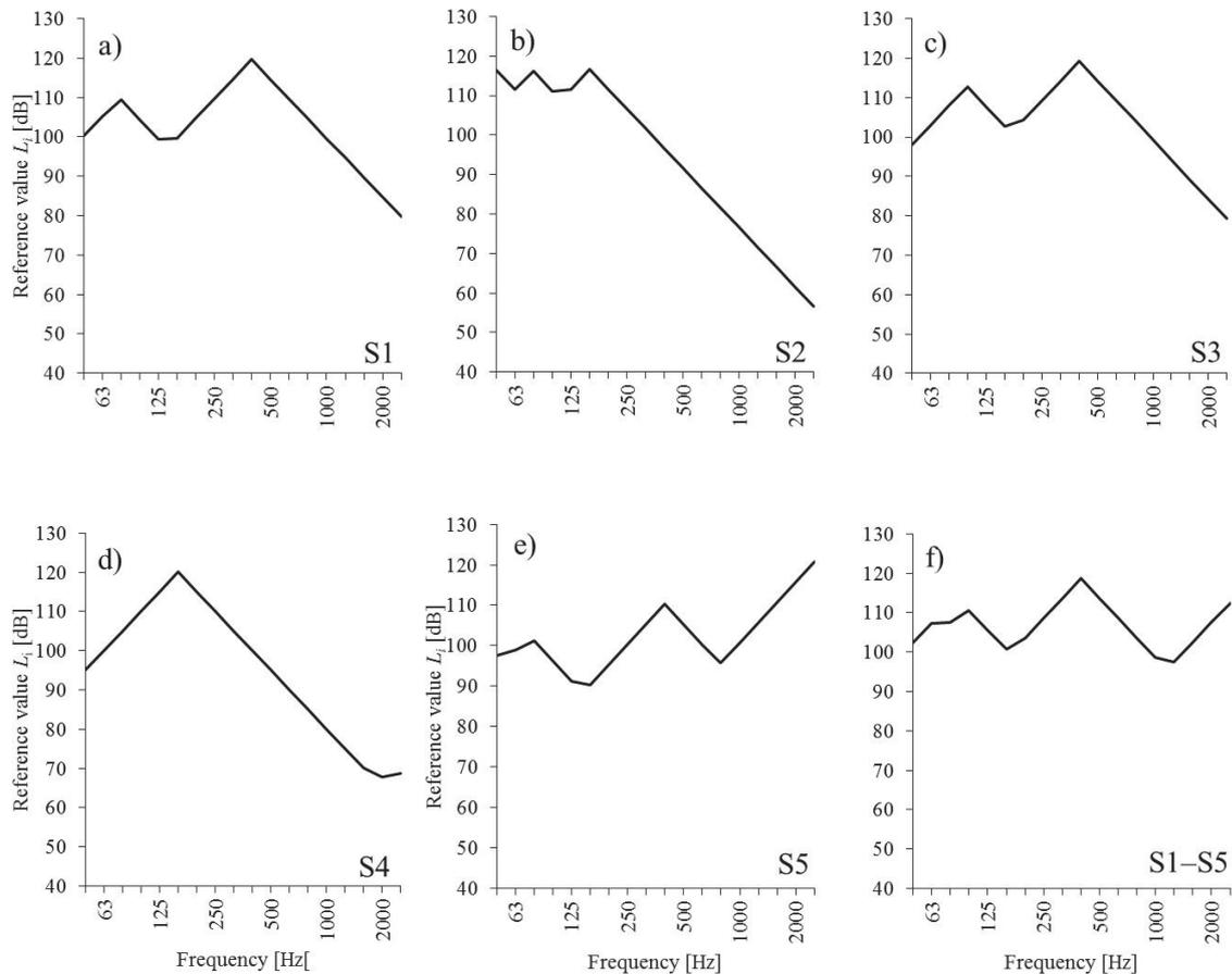
Figure 3 – The sound type optimized reference spectra  $L_{S1} \dots L_{S5}$  for the impact *sound types* S1–S5 (panels a–e) and the optimized reference spectrum  $L_{opt}$  for all sound types S1–S5 (panel f).
