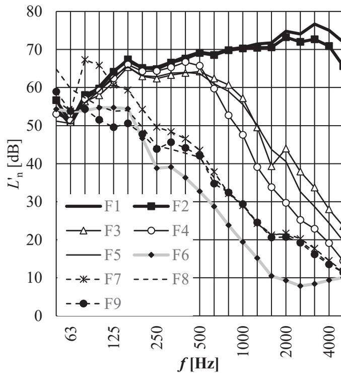
Figure 2 – Measured normalized impact sound pressure levels  $L'_n$  of the nine floor types F1–F9.
