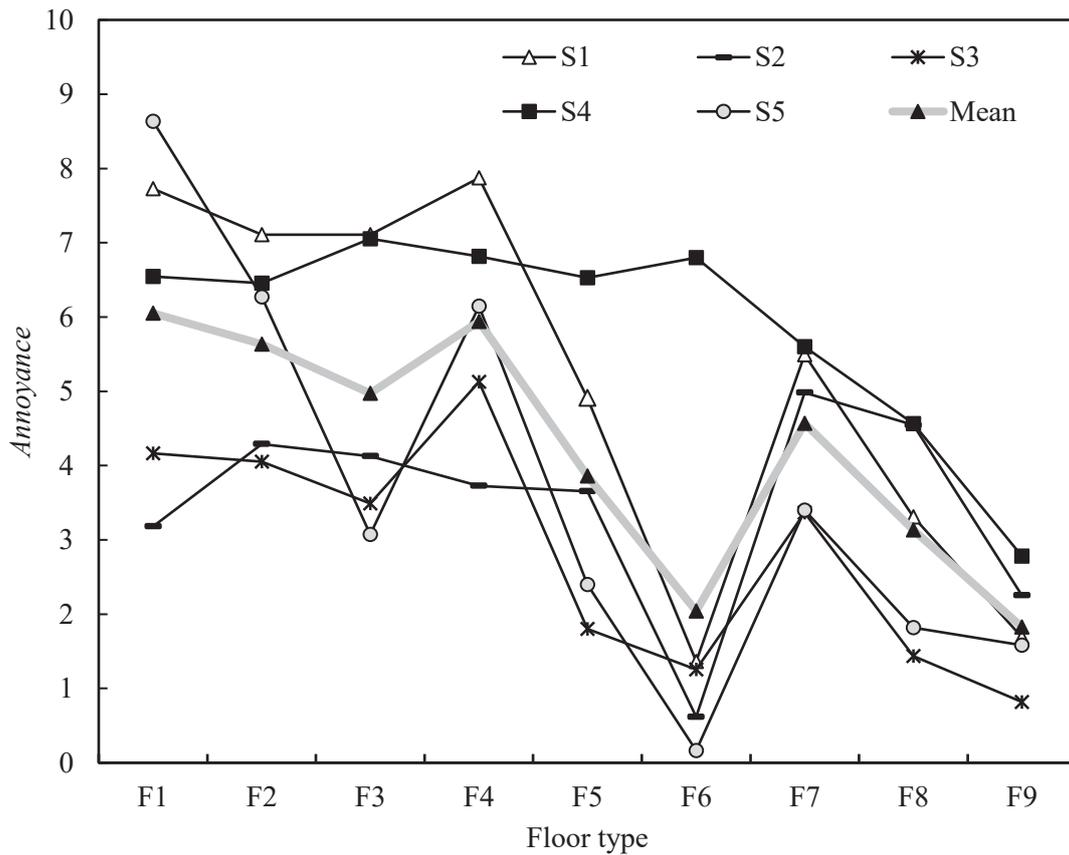
Figure 1 – Mean values of subjective annoyance for each combination of impact sound types S1–S5 and floor types F1–F9. In addition, the mean over all five sound types (Mean) is shown. The variable on the X-axis is categorical. Lines are used to facilitate the reading of data.
