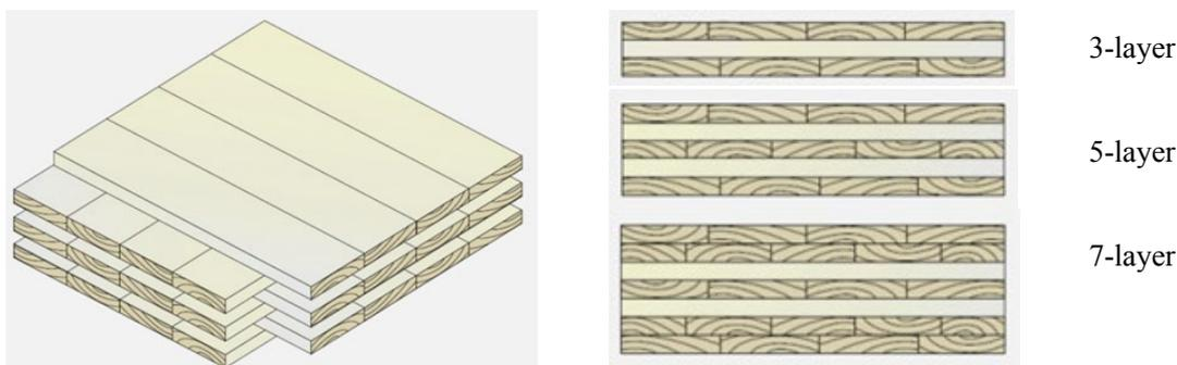
Figure 1 – Example of CLT panels.
