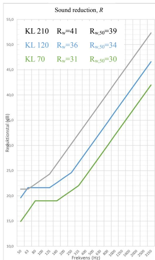
Figure 3 – Sound reduction for CLT panels of three thicknesses; 70, 120 and 210 mm.
