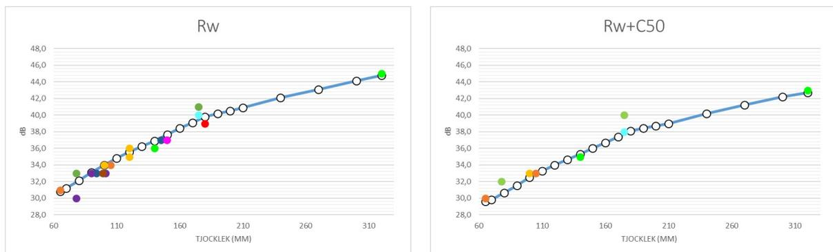
Figure 4 – Single number ratings of CLT panels. Open circles are predicted values and filled colored circles represent verifying data from various references.
