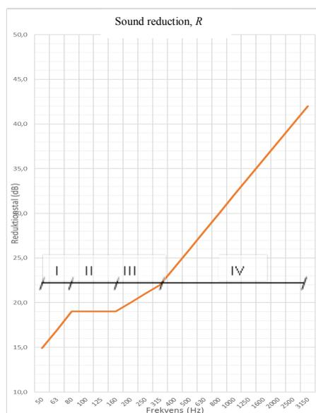
Figure 2 – The sound reduction model is divided into four frequency regions.
