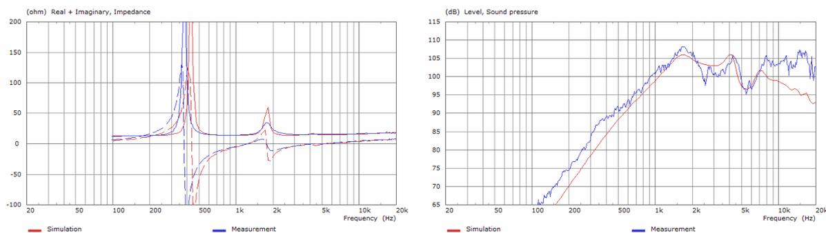
Figure 12 - Simple model: Electric driving point impedance and sound pressure level at 180 mm on-axis in front of aperture
