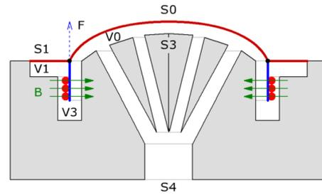
Figure 3 - Compression driver cut-view
