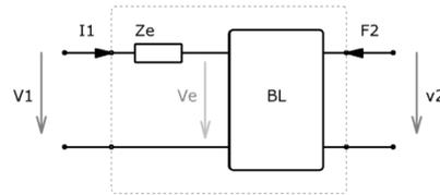
Figure 5 - Electro dynamic motor
