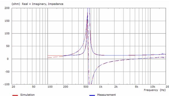
Figure 7 - Electrical driving point function of driver in vacuum
