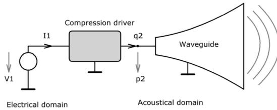
Figure 2 - Electro-acoustic transducer
