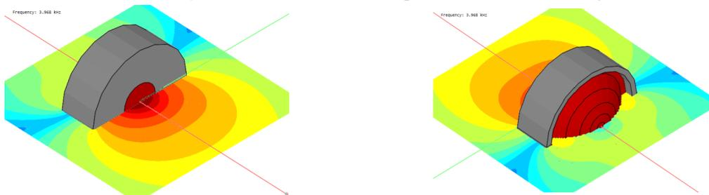
Figure 10 - Free radiation. Example of pressure field at 3900 Hz (range 50 dB).
