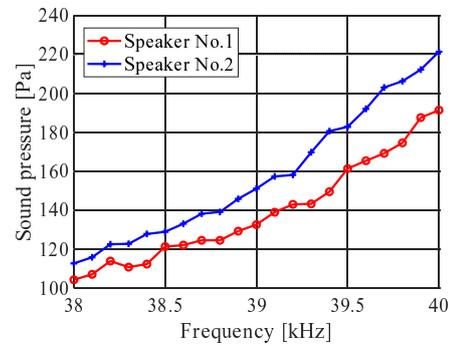
Figure 2. Frequency - sound pressure characteristics of speakers when input voltage is  $2 V_{pp}$ .
