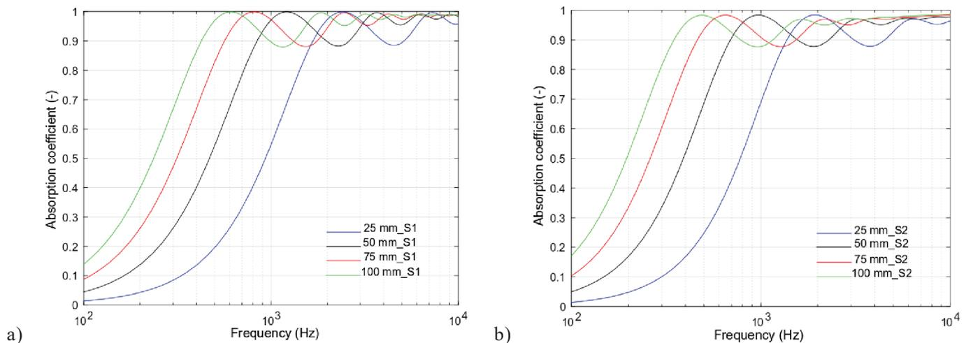
Figure 4 –Absorption coefficients as a function of different thickness of sample for S1 (a) and S2 (b) sample
