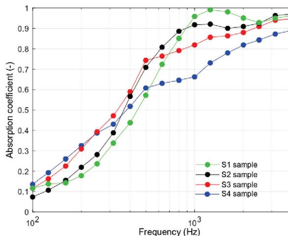
Figure 2 - Normal incidence absorption coefficients of the investigated materials
