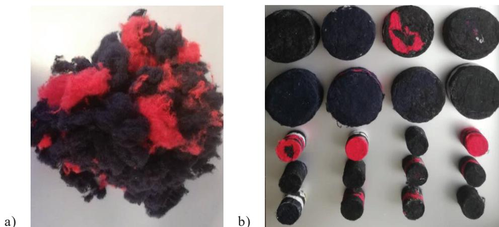
Figure 1 – Wool batting matrix (a) and woolen innovative composite materials (b)
