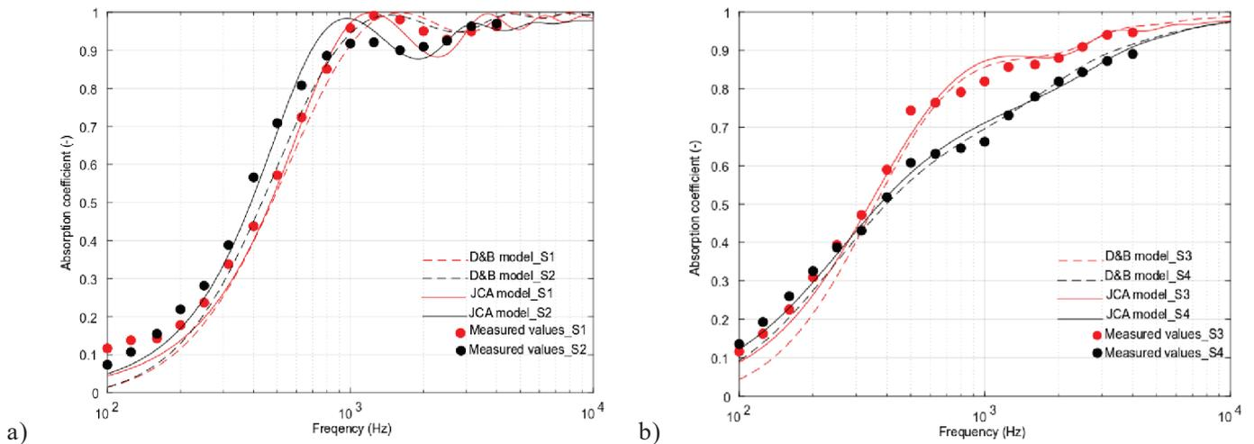
Figure 3 – Normal incidence absorption coefficients of S1, S2 samples (a) and of S3 and S4 samples (b)
