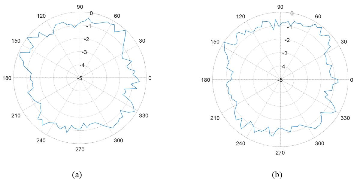
Figure 3 – Beam patterns of an ultrasound source. (a) On a horizontal plane (base plane of cleaner). (b) On a 60° cone with the apex at the acoustic center of the source.
