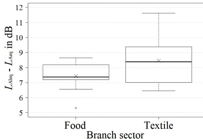
Figure 2. Boxplot: difference between  $L_{A_{Ieq}} - L_{A_{eq}}$  in cashiers area for stationary measurements with arithmetic average “×” and an outlier “o” from 22 stationary measurements in food and 18 in textile retail.
