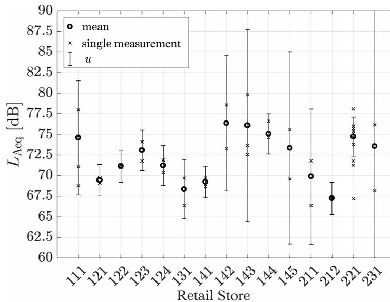
Figure 1. Evaluation of single measurements  $L_{Aeq}$  as energy-equivalent mean per retail store (code for anonymity) with combined standard uncertainty  $u$  according to [3] and single measurements “×”.
