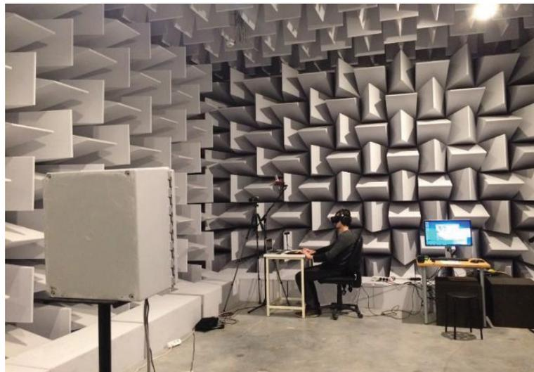
Figure 1 – Experimental setup for virtual reality experiment in the semi-anechoic room.
