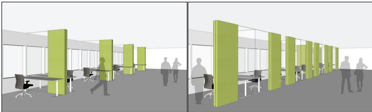
Figure 2 – Illustration of room-high I-shaped sound screens (left) and T-shaped sound screens (right)
