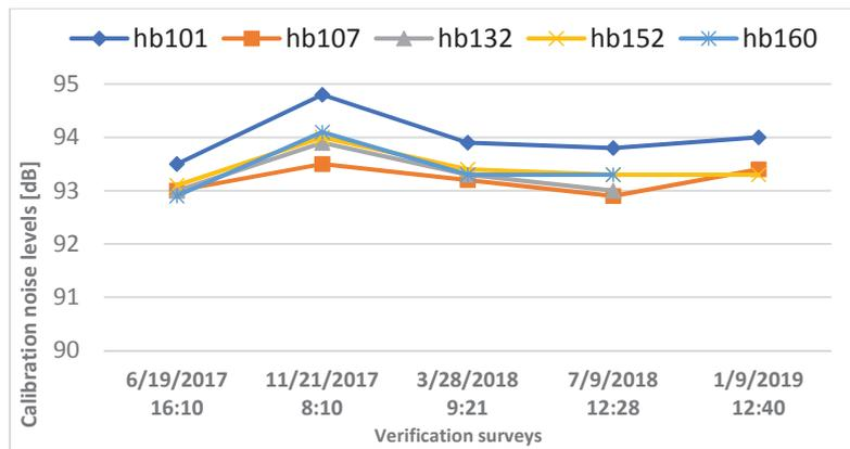
Figure 4– 1 kHz calibration check – Electret sensors placed on building’s façades.
