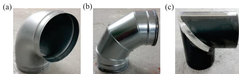
Figure 5 – Tested bended elements: (a) rounded bend, (b) bend by straight parts, (c) sharp bend.
