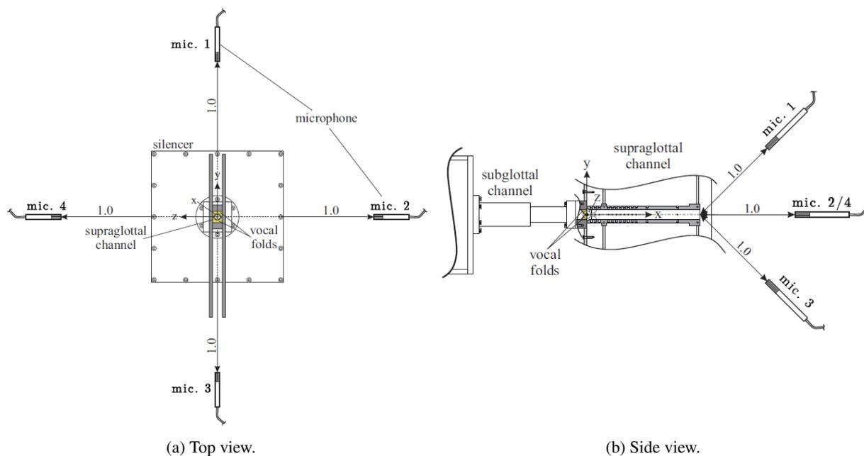
Figure 3. Schematic of the experimental setup for sound measurements of vibrating vocal folds. All dimensions in m. Extracted from [7].
