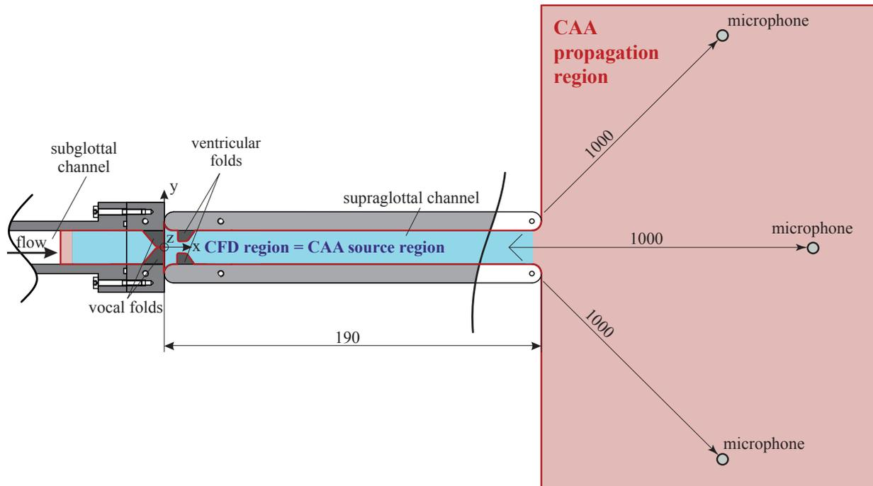
Figure 1. Schematic of the larynx model: subglottal, glottal, supraglottal regions, and the sound propagation region with microphone positions. The CFD (bluish) and the CAA (reddish) geometry is adapted to the experimental setup. All dimensions are in mm. Extracted and modified from [7].
