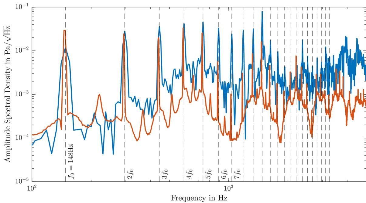
Figure 4. Comparison of the amplitude spectral density of the simulation results (blue) and measurement results (orange).
