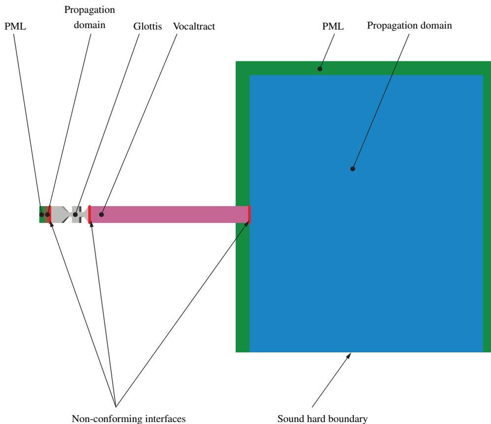
Figure 2. Geometry and mesh of the acoustic simulation: subglottal, glottal, supraglottal region, the sound propagation region, and the perfectly matched layer (PML) regions.
