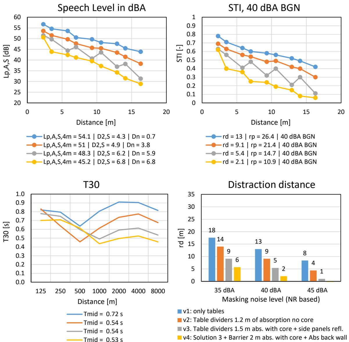
Figure 5: measurement results for four different variations of furniture setups
