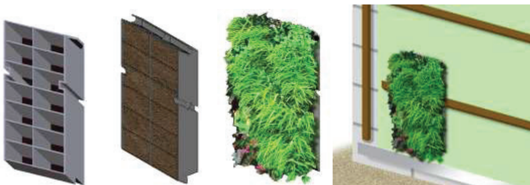
Figure 2 - Living Green Wall schematics (11), left-to-right: single empty module, module with soil, module with plants, attached module to the LGW construction wall
