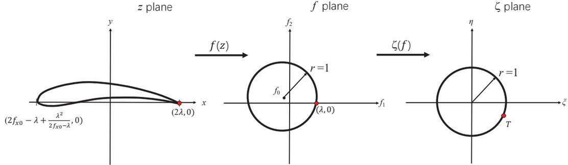
Figure 2. Successive mappings of a generalized Joukowski airfoil in the physical  $z$ -plane to a unit circle centered at the origin in the  $\zeta$ -plane,  $T$  is the trailing edge location. The trailing-edge position through the successive mappings is indicated by the red dot.
