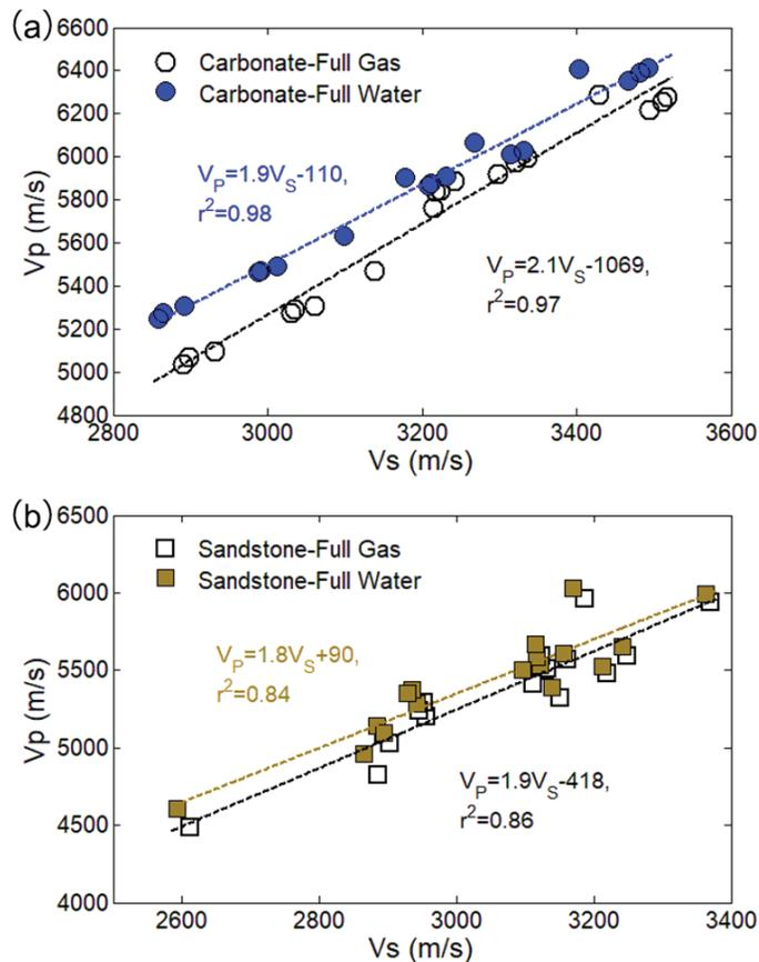
Figure 1. Crossplots of  $V_p$  and  $V_s$  for (a) 18 carbonates and (b) 17 sandstones at full gas and full water saturations. Linear fits are shown.
