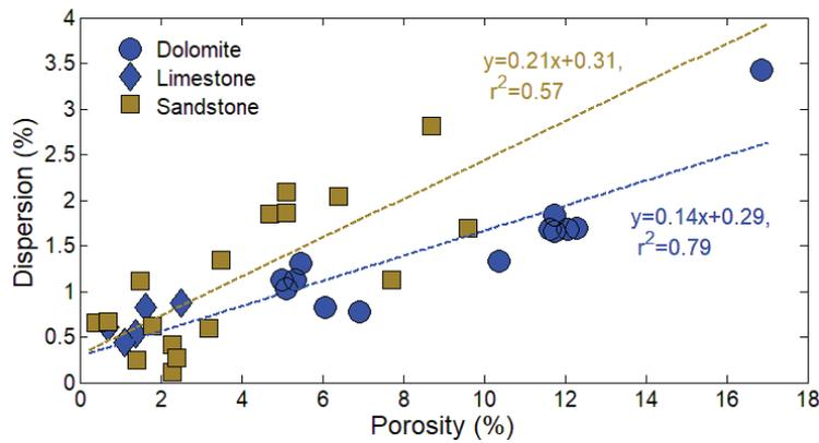
Figure 2. Crossplot of P-wave velocity dispersion and porosity for the tight carbonates (including dolomites and limestones) and sandstones in our measurements. The dashed linear represent the regressions.
