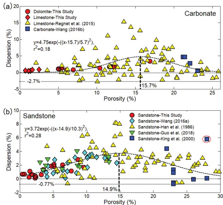
Figure 3. Crossplots of P-wave dispersion and porosity for the whole datasets of (a) carbonates and (b) sandstones. Gaussian fits are shown.
