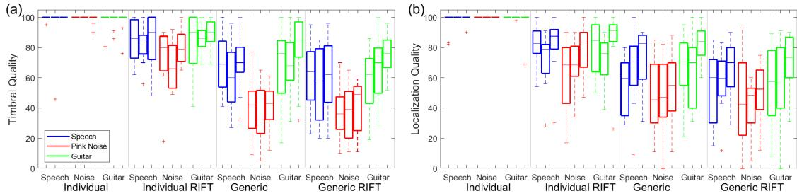
Figure 6. Ratings for all test conditions. Ratings are grouped by HRTF type and stimulus as indicated in the labels. For each group three tested directions are presented: left to right -  $[60^\circ, 0^\circ]$ ,  $[60^\circ, 30^\circ]$ ,  $[-15^\circ, 45^\circ]$ . The box bounds the interquartile range (IQR) divided by the median, and Tukey-style whiskers extend to a maximum of 1.5IQR beyond the box [13]. Ratings for (a) *Timbre quality* (b) *Localization quality*
