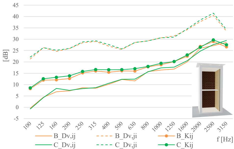
Figure 6 – D_{v,ij(ji)} and K_{ij} for the “L vertical junction” transmission path measured in B and C solutions.
