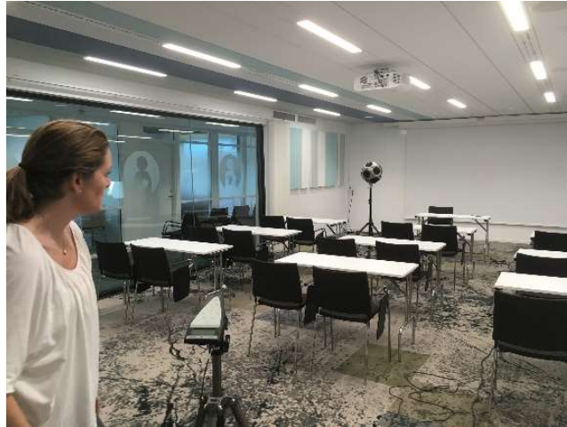
Figure 5 – Config. 4. Now with the additional 7.2m 2 of wall absorbers distributed over three walls
