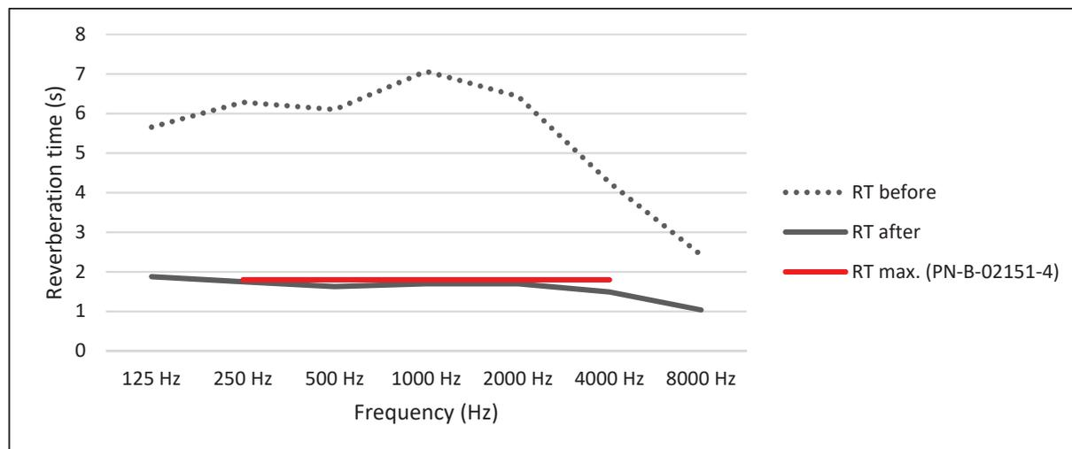
Figure 2 – Sport hall, reverberation time RT, (s), before and after acoustic treatment
