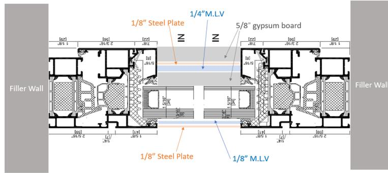
Figure 2 - Drawing detail of the masked window
