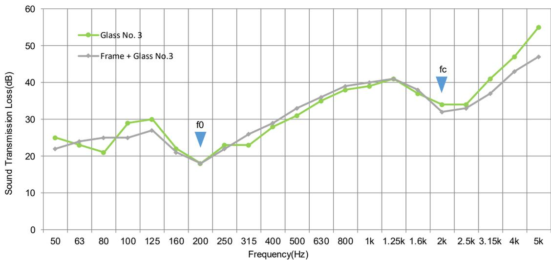
Figure 3 - STL of unframed and framed double insulating glass No. 3
