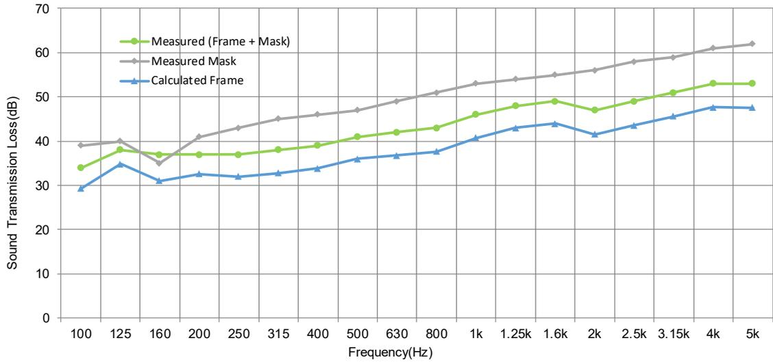
Figure 6 - STL of measured framed mask system, unframed mask composite, and calculated frame results
