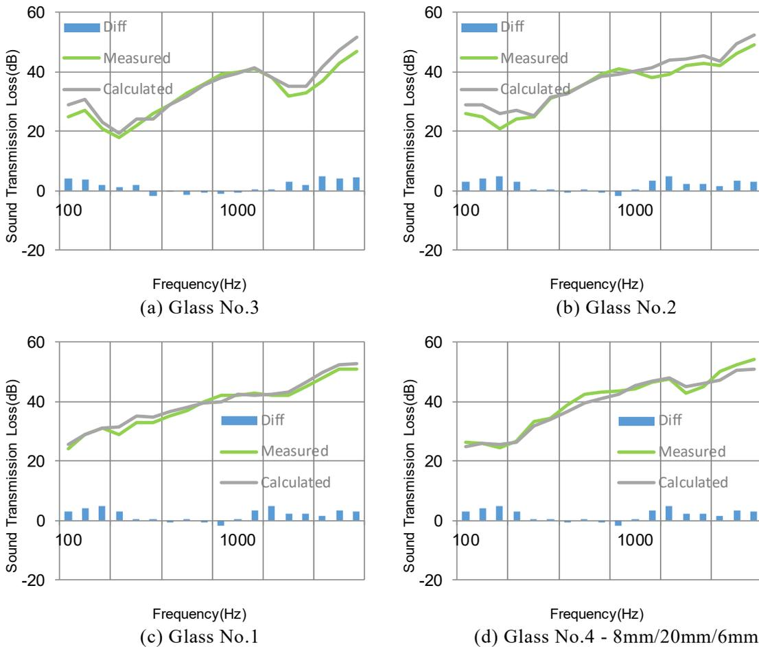
Figure 7 - STL comparison of measured and predicted window results of four different glass options
