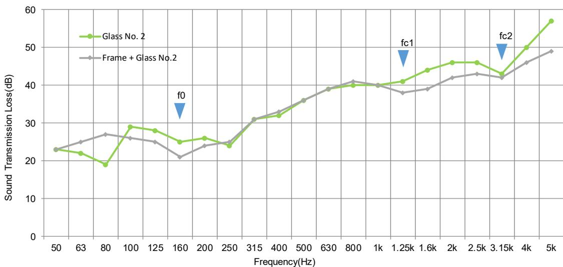
Figure 4 - STL of unframed and framed double insulating glass No. 2
