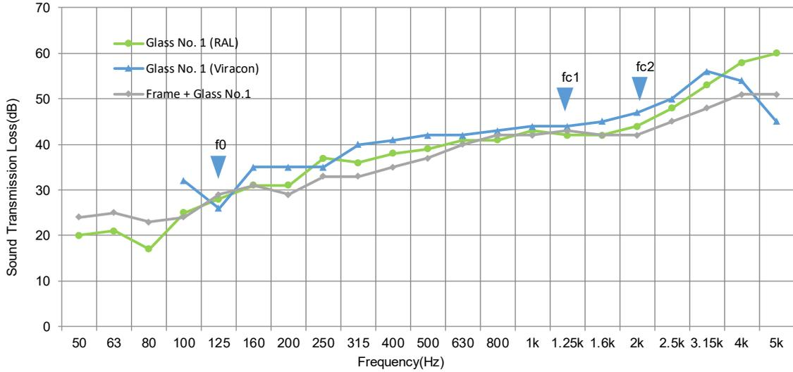
Figure 5 - STL of unframed and framed double laminated glass No. 1
