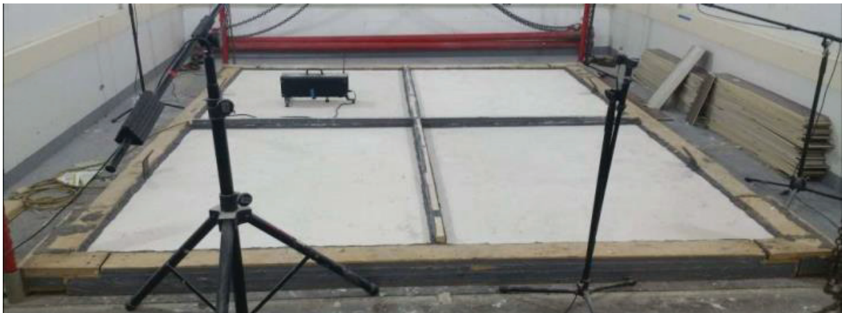
Figure 1 – A picture of the top surface of the assembly divided into 4 Floor Zones. A different floor topping will be installed in each Floor Zone.
