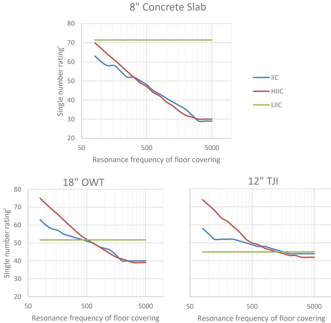
Figure 2 – Single number ratings as a function of resonance frequency of theoretical floor covering behaving as Eq. (1) for three structural systems: 200 mm concrete slab (top), 457 mm open web wood trusses (bottom left), and 300 mm wood I-joists (bottom right).
