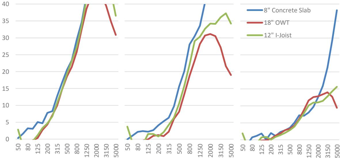
Figure 1—Improvement in impact insulation (reduction in impact sound level) on three structural systems for carpet tile (left), luxury vinyl plank over foam mat (middle), luxury vinyl plank without sound mat (right).
