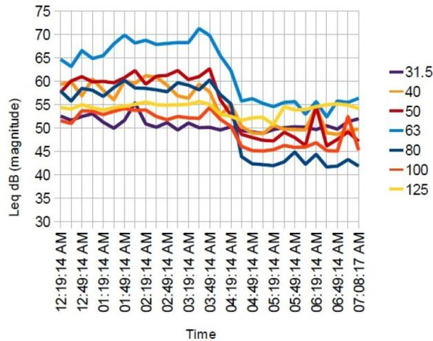
Figure 1: Third octave band measurements of Leq in a bedroom on 5<sup>th</sup> floor of condominium above an open stairwell with club on 1<sup>st</sup> floor, Note the drop in level of 15dB when the club closes at 4:00am.
