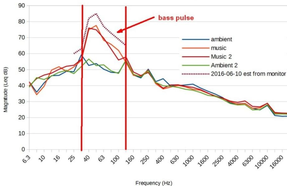
Figure 2: Outdoor measurements 29m (95ft) from a club in an apartment complex 12:00am versus ambient conditions.
