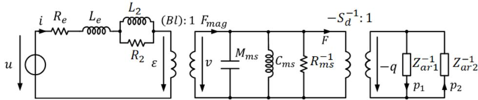
Figure 1. Equivalent circuit representation of the voice coil loudspeaker mounted in a baffle;  $\epsilon = -Blv$  is the back electromotive force,  $F_{mag} = Bli$  is the magnetic force on the current-carrying wires, and  $q$  is the volume velocity.
