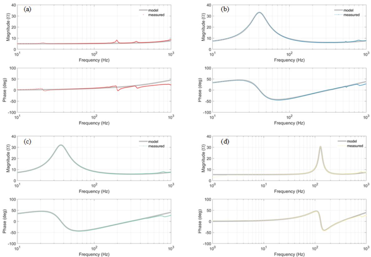
Figure 3. Measured and fitted data of the electrical impedance of the loudspeaker driver (a) when the coil is blocked, (b) in vacuum, (c) mounted in a baffle in anechoic chamber and (d) closed-box loudspeaker mounted in a baffle in anechoic chamber.
