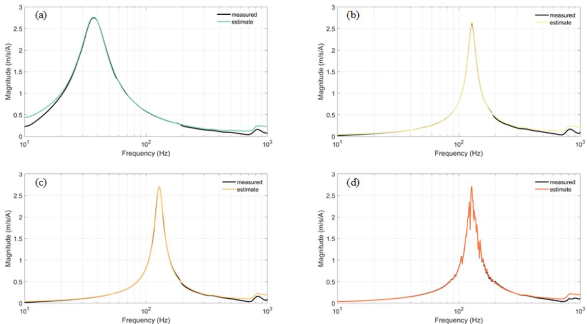
Figure 5. Frequency response function between the input current and the output velocity as given in Eq. (4) of (a) the loudspeaker mounted in a baffle in anechoic chamber, (b) the closed-box loudspeaker mounted in a baffle in anechoic chamber, (c) the closed-box loudspeaker placed in an anechoic room and (d) in a lightly damped room.
