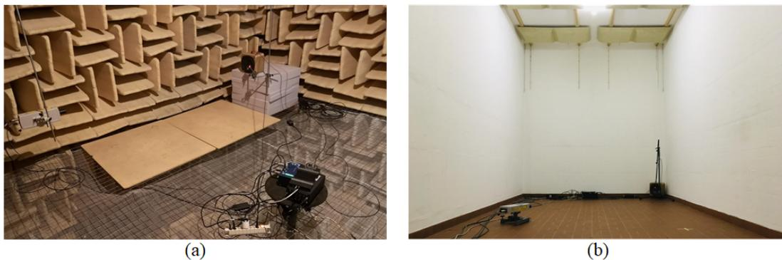
Figure 4. Experimental setup for estimating the front-side acoustic load impedance on the closed-box loudspeaker system (a) placed in an anechoic room and (b) located near a corner in a lightly damped room.
