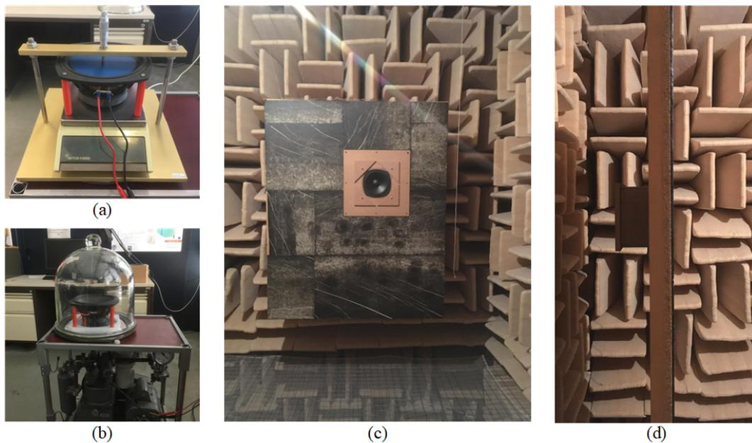
Figure 2. Experimental setup for measurement of the electrical impedance of the loudspeaker driver (a) when the coil is blocked, (b) in vacuum, and (c) mounted in a baffle in open space. In (a), a specific locking system is used to prevent the diaphragm from vibrating, and thus the coil attached thereto; in (b), the loudspeaker driver unit is placed in a vacuum chamber to eliminate the effect of air on the diaphragm; in (c), the loudspeaker driver is mounted in a baffle in an anechoic chamber.
