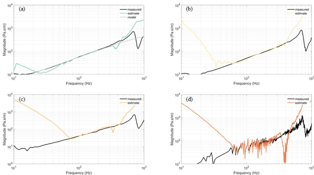
Figure 6. Frequency response function of the specific acoustic impedance (see Eq. Eq. (5)) of (a) the loudspeaker mounted in a baffle in anechoic chamber, (b) the closed-box loudspeaker mounted in a baffle in anechoic chamber, (c) the closed-box loudspeaker placed in an anechoic room and (d) in a lightly damped room.
