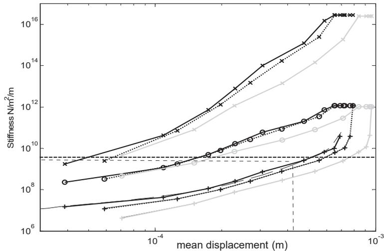
Figure 8- Contact stiffness v mean displacement  $\bar{w}_n$ , — single profile, ..... triple profile, — full profile, x---x bending, o---o tension-shear, +---+ indentation, - - - tread block, - - - fit to full profile
