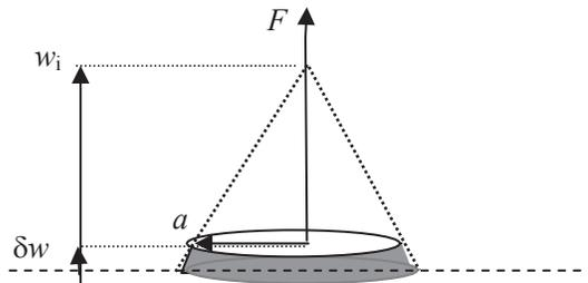
Figure 2- Indentation into a half-space for a general profile
