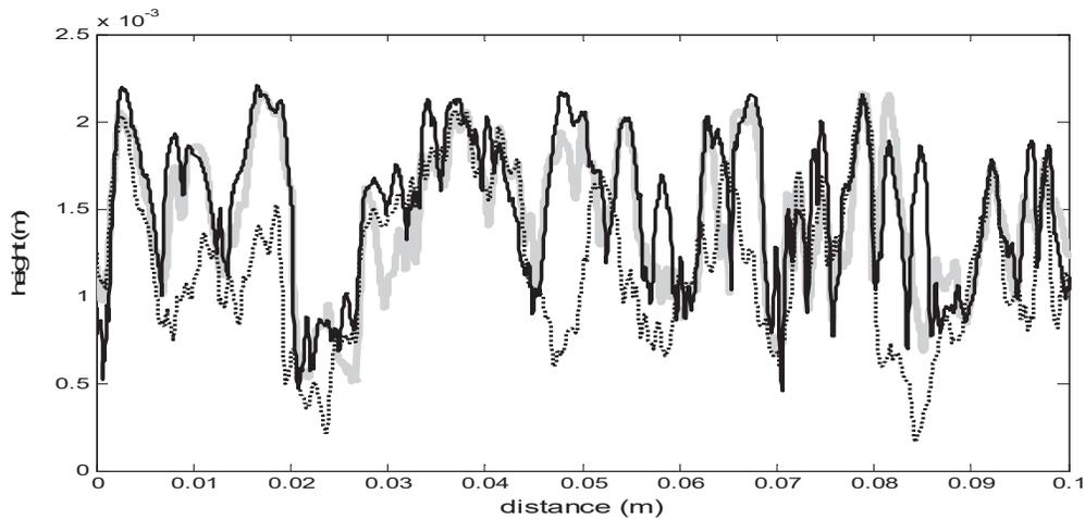
Figure 6- Road profiles: ..... single profile, — triple profile, — full profile
