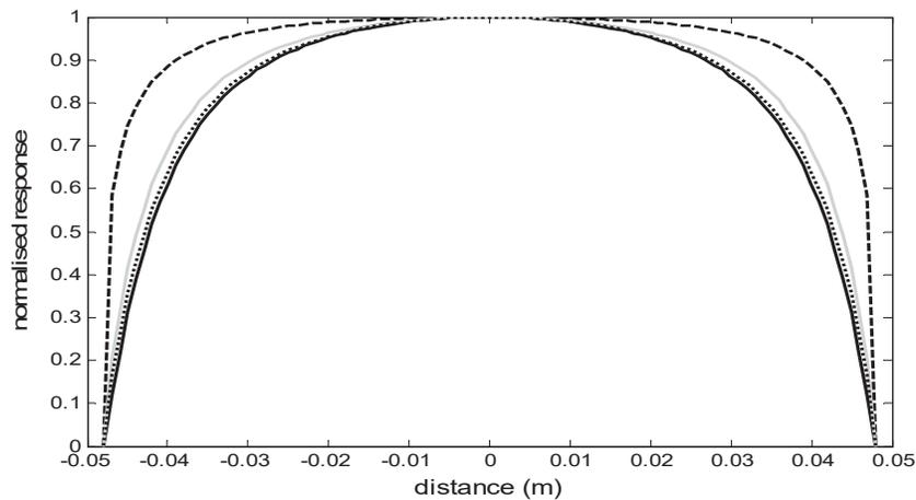
Figure 11- Pressure, stiffness and displacement of the tyre contact patch: \_\_\_\_\_  $p_s$  static pressure normalised to  $p_{s0}=1.8 \times 10^5 \text{N/m}^2$ , - - -  $w_s$  static envelope normalised to  $w_{s0}=0.415 \text{mm}$ . .....  $K_d$  dynamic stiffness normalised to  $K_{d0}=1.5 \times 10^9 \text{N/m}^2/\text{m}$ , ———  $K_s$  static stiffness, normalised to  $K_{s0}=4.25 \times 10^8 \text{N/m}^2/\text{m}$
