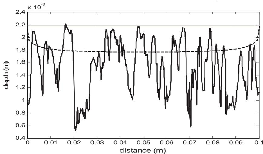
Figure 13- Displacement profiles in the contact patch: — strip profile  $w_N$
