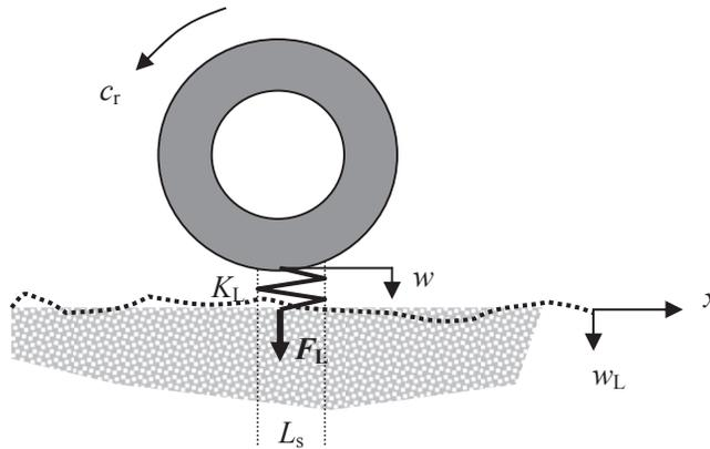
Figure 12- Long wavelength excitation of a rolling tyre
