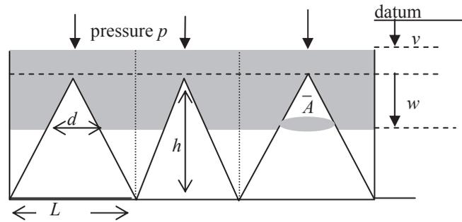
Figure 3- Diagonal section through an array of identical particles
