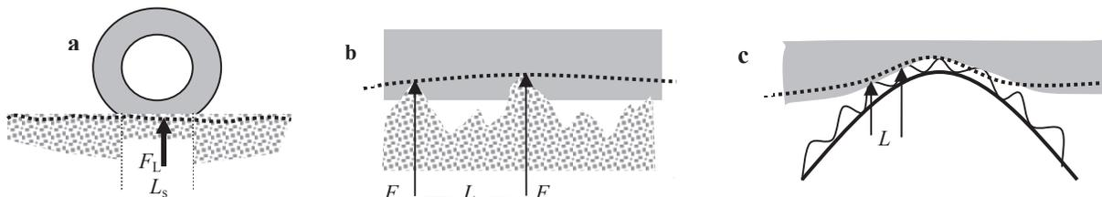
Figure 1- Contact between a tyre and a road surface: ..... peak envelope,
