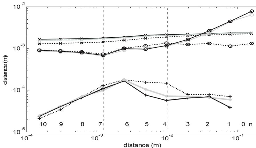
Figure 7- Mean profile properties v level  $n$ : ..... single profile, ——— triple profile, ——— full profile: x---x envelope, +----+ step; o-----o contact diameter .
