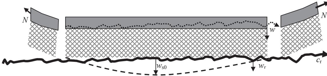
Figure.10- Section of a one-dimensional tyre in rolling contact with a road
