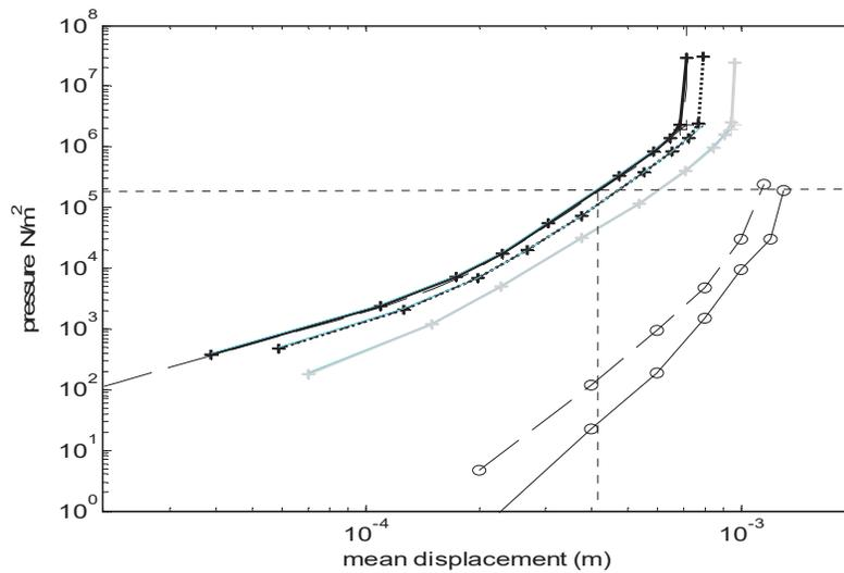
Figure 9- Contact pressure v displacement  $\bar{w}_n$ , — single profile, ..... triple profile, — full profile, o---oconcrete surface (6), σ—o asphalt surface (6), - - - - fit to full profile
