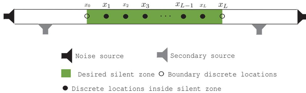
Figure 5. Scheme of acoustic simulated system.
