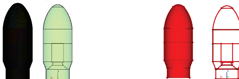
Figure 7 - FE model and SEA model Figure 8 - Point, line and surface connections of payload/fairing combination
