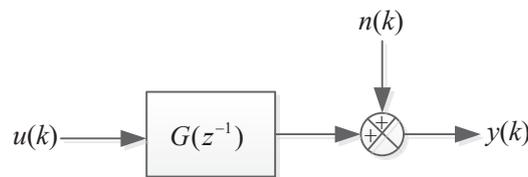
Figure 3 – A general SISO system with disturbance
