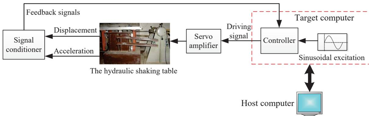
Figure 1 – The whole shaking table system
