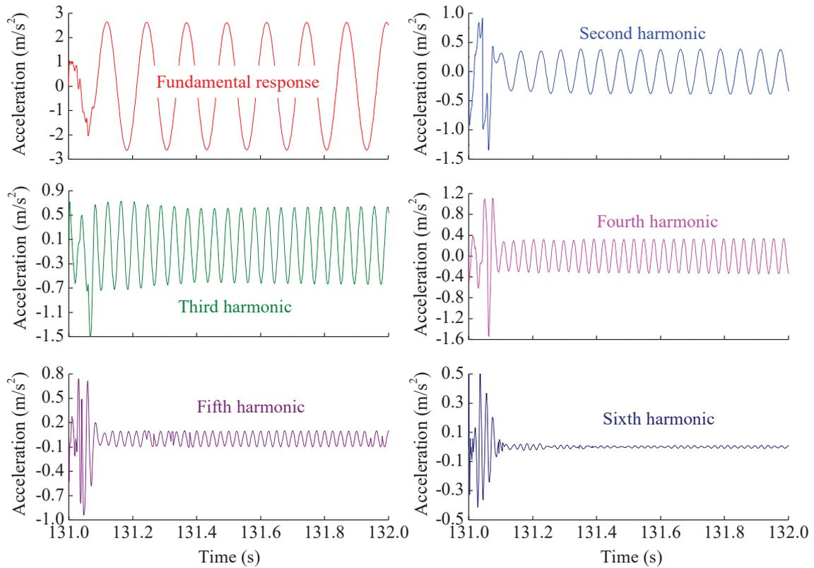
Figure 8 – The waveform of each harmonic component
