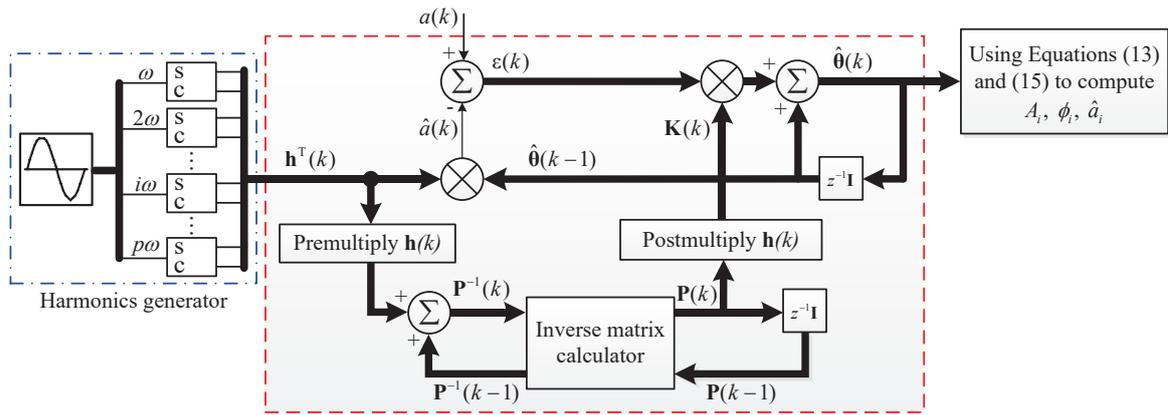
Figure 5 – Acceleration harmonics identification scheme
