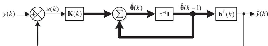
Figure 4 – Block diagram of the RLS algorithm
