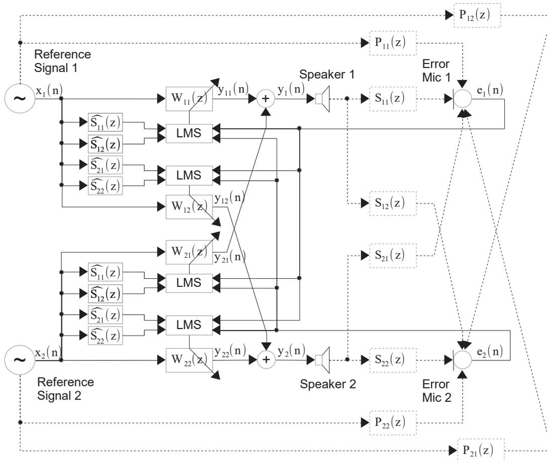
Figure 4 – 2 x 2 x 2 MIMO system, utilizing the MEFXLS algorithm, shown in more detail
