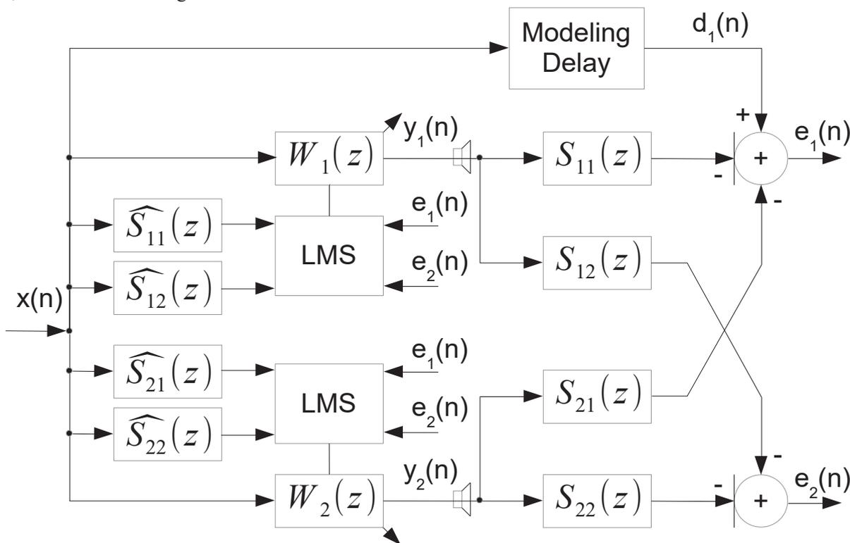
Figure 3 – Modified MEFXLS algorithm for the creation of individual sound zones (bright zone at error microphone 1 ( $e_1(z)$ ) and a dark zone at error microphone 2 ( $e_2(z)$ ))
