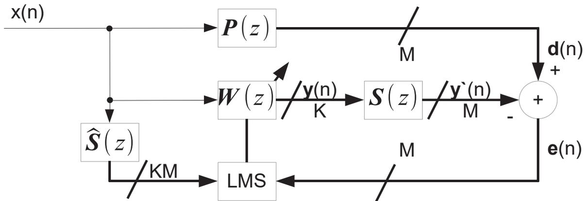
Figure 1 - Generalized  $1 \times K \times M$  MIMO system, utilizing the MEFXLMS algorithm
