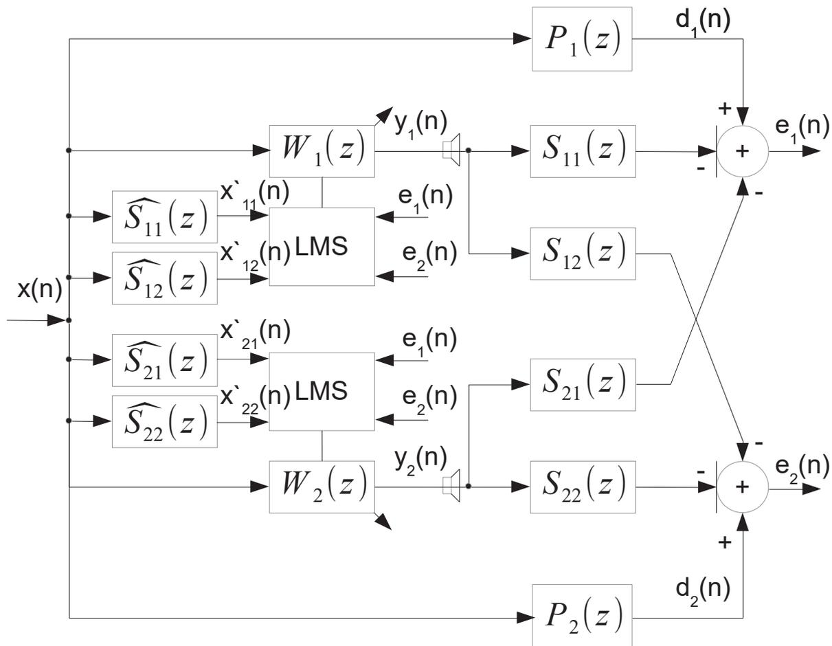
Figure 2 –  $1 \times 2 \times 2$  MIMO system, utilizing the MEFXLMS algorithm
