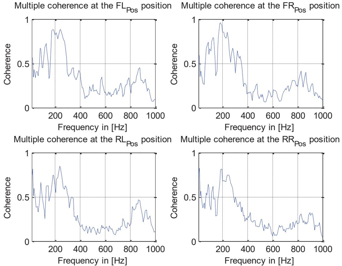
Figure 6 –MCA at all four seat positions, where the corresponding error microphones had been installed, utilizing the following ACC sensor signals:  $FL_{SubY}$ ,  $FL_{SubZ}$ ,  $FR_{SubY}$ ,  $FR_{SubZ}$ ,  $RL_{HubY}$ ,  $RL_{HubZ}$ ,  $RR_{HubY}$ ,  $RR_{HubZ}$  for the calculation of the multiple coherence.
