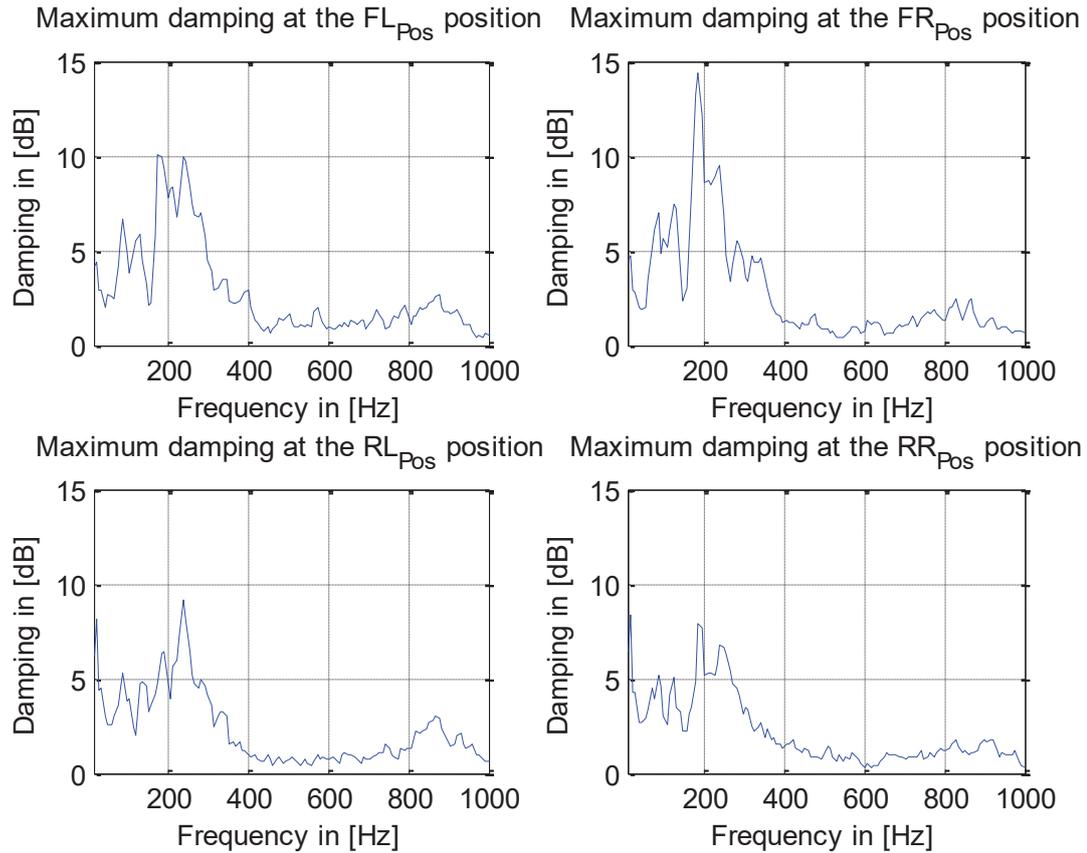
Figure 7 – Damping performance at all four seat positions, as predicted by the MCA.
