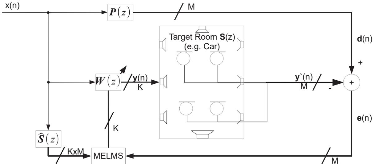
Figure 5 – 1 x 2 x 2 MIMO system, utilizing the MEFXLS algorithm, shown in more detail
