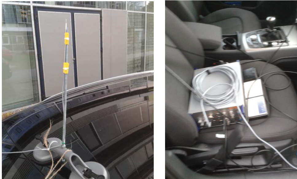
Figure 6 – SVM Data acquisition system; flow sensor (left), frontend (right)
