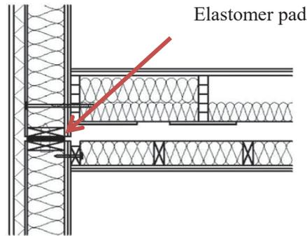
Figure 2 - Elastomer flanking couplings for decoupling of floor from the supporting structure, construction type B: Elastomer isolator pads loaded by whole room volume units.
