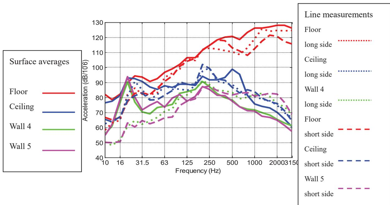
Figure 10 - Acceleration levels caused by an impact hammer machine. Comparison between the measured line of 5 points 0,2m from the flanks and complete surface average measurements.
