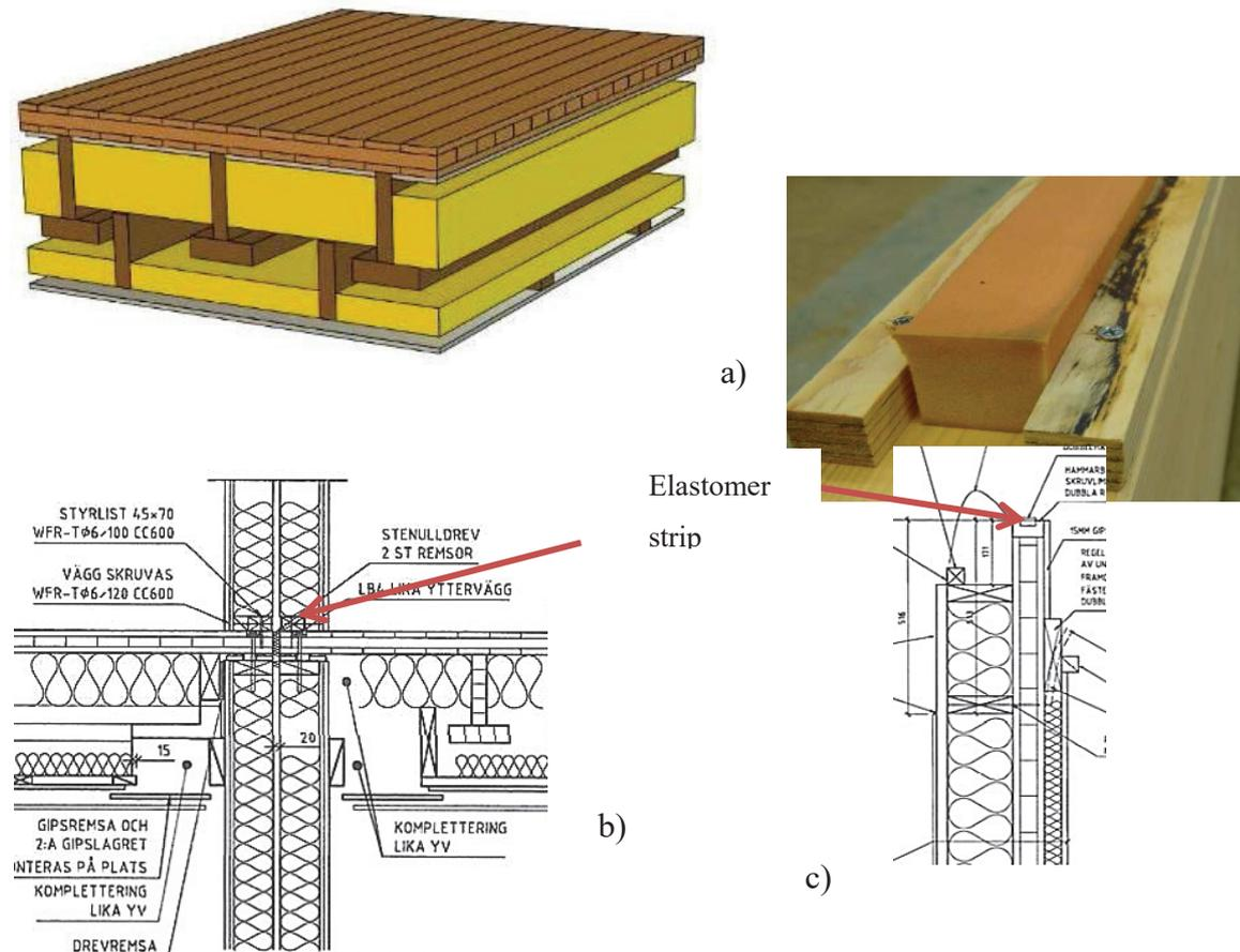
Figure 1 - Elastomer flanking couplings for decoupling of the floor from the supporting structure, type A: a) Separate CLT floor and ceiling. Elastomer strips loaded by the floor cassette. b) Coupling for apartment separating walls. c) Outer wall with a CLT load bearing wall plate and a radiation protection isolating layer.
