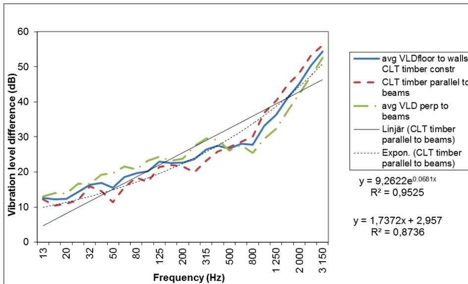
Figure 4 - Comparison of vibration level difference over the flanks from floor to wall in two directions; perpendicular to and parallel with the load bearing beams. Construction type A, CLT plate and beams with line elastomer strips. Average for five floors.
