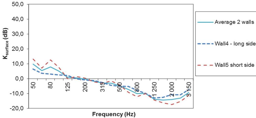
Figure 11 - Surface average compensation factor  $K_{surface}$  measured for two walls.
