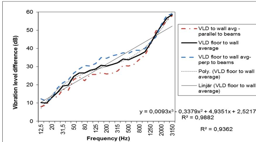
Figure 5 - Vibration level difference over the flanks from floor to wall in two directions; perpendicular to and parallel with load bearing floor beams. Construction type B, three objects. Elastomer pads.
