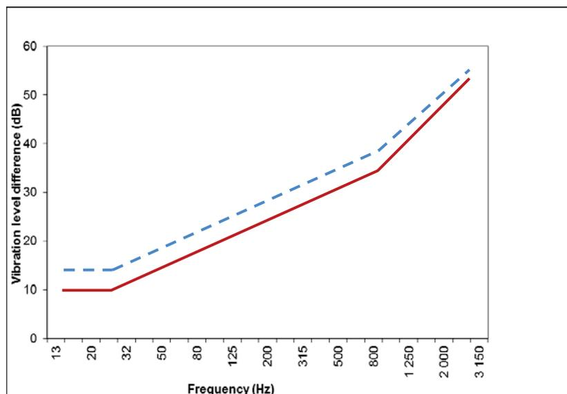
Figure 8 - Generalized average vibration level difference over the flanks from an impact excited floor to the receiving walls, for two floor construction types with elastomers.
