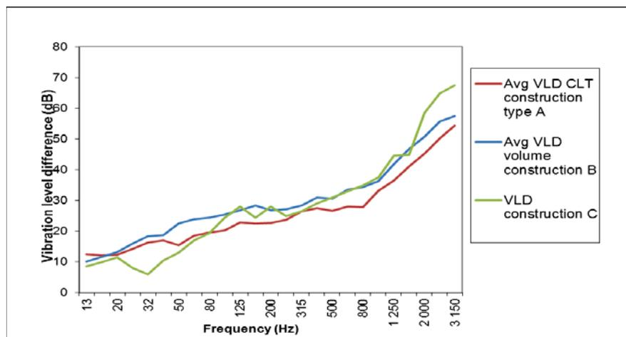
Figure 7 – Average vibration level difference over the flanks from an impact excited floor to the receiving walls. Comparison between three floor construction types.
