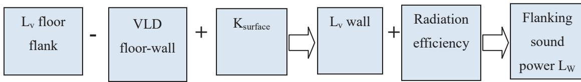
Figure 9 - Principle drawing of how the VLD can be used for determination of flanking contributions.
