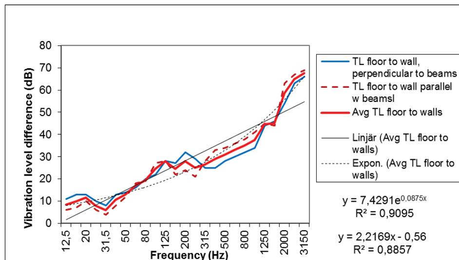
Figure 6 - Vibration level difference over the flanks from floor to walls. Comparison of VLD perpendicular to the beams and parallel with the beams. Construction type C. Only one object.
