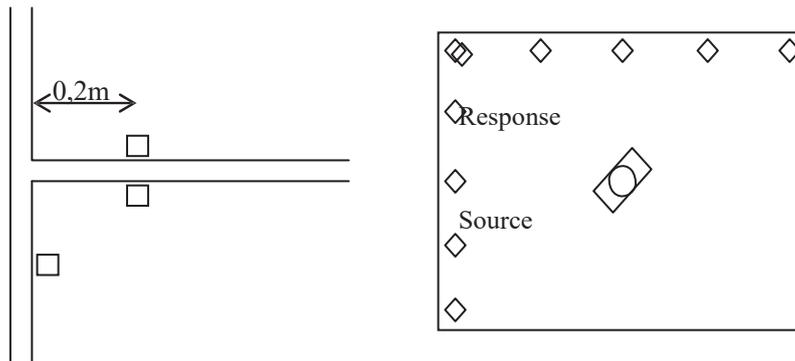
Figure 3 - Accelerometer positions for the simplified flanking transmission vibration level difference, VLD, field measurements. Five accelerometers along each line.
