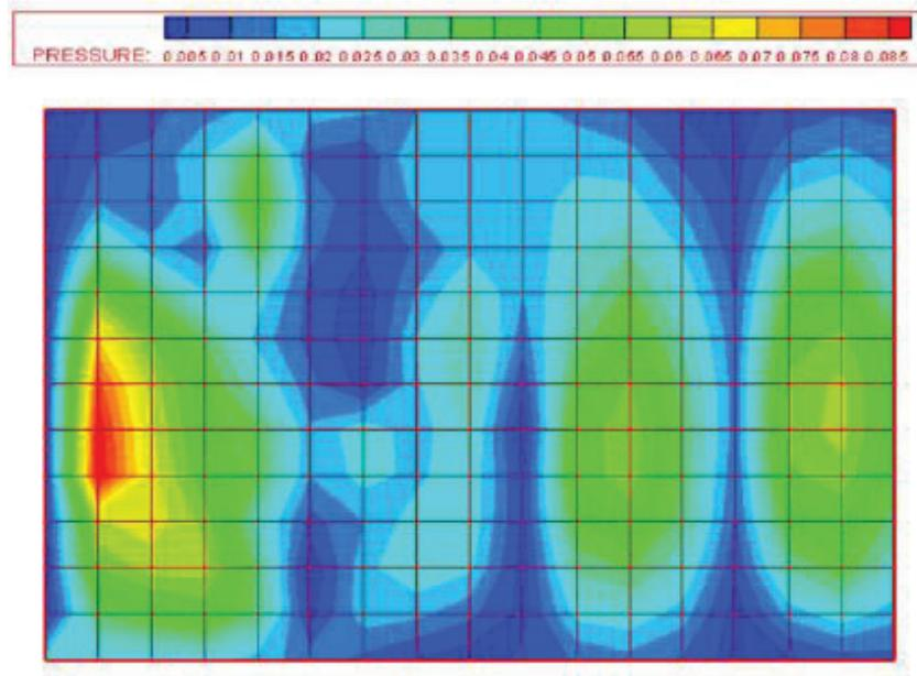
Figure 5 – The surface pressure obtained by modified Green function.
