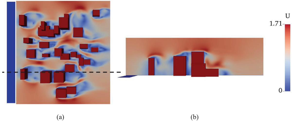
Figure 1 – Instantaneous contours of the velocity magnitude taken from the LES simulation. Note that the solid blue rectangle indicates the position of the road. (a) Contour in the x-y plane at z=1m. (b) Contour in the x-z plane, plotted at the location indicated by the dashed line in figure 4(a).
