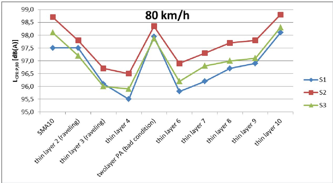
Figure 4 – L<sub>CPX:P,80</sub> values for three tyre sets on 10 different pavements at 80 km/h.
