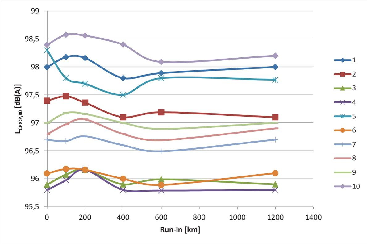
Figure 1 -  $L_{CPX:P,80}$  as a function of kilometers run-in for 10 various test sections for P1 tyre at 80 km/h.
