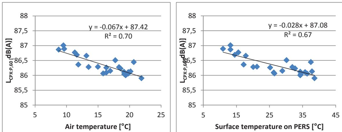
Figure 6 –  $L_{CPX:P,60}$  levels as a function of air temperature (left) and surface temperature (right).
