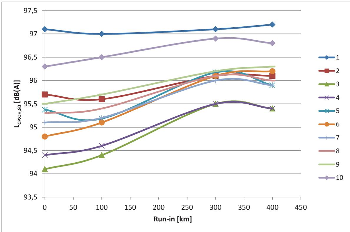
Figure 2 -  $L_{CPX:H,80}$  as a function of kilometers run-in for 10 various test sections for H1 tyre at 80 km/h.
