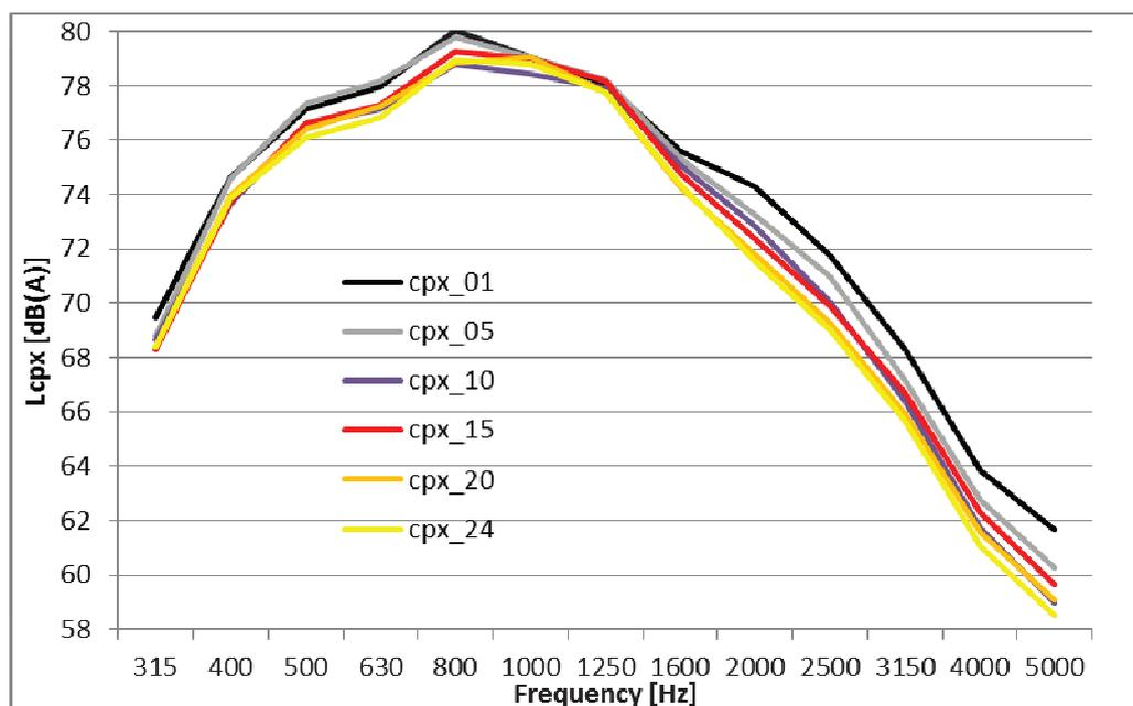
Figure 7 - Frequency spectra of six various measurements (01 to 24 from low to high temperature).
