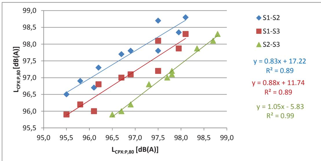
Figure 5 – Correlation between various tyre sets Sx-Sy at 80 km/h. The first mentioned tyre set is each time positioned on the horizontal axis.
