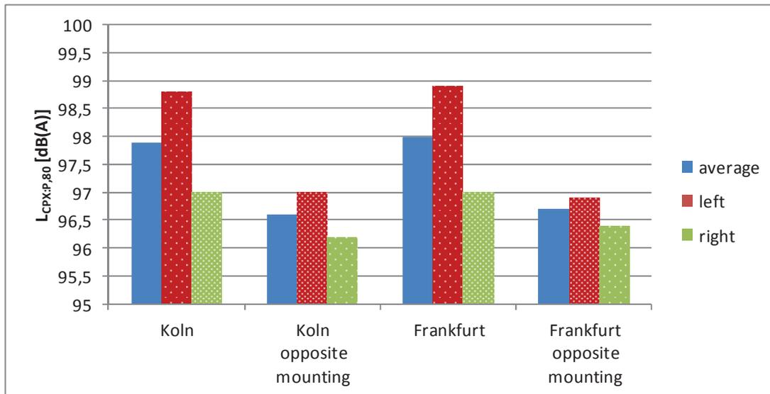
Figure 3 –  $L_{CPX;P,80}$  of S3 (average, left and right tyre) at 80 km/h. The measurement direction is given on the horizontal axis. The pattern fill (dots) indicates the tyre which was used (left/right).
