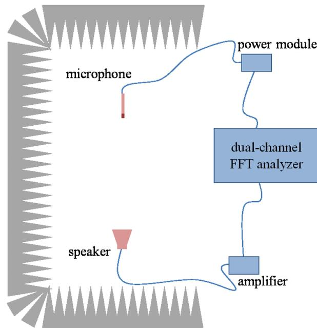
Figure 1 – Sketch of set-up in free-field environment
