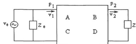
Figure 1 – Electro-acoustic analogy circuit
