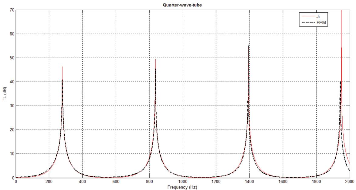
Figure 8 – Transmission loss comparison between 1D analytical model with Ji's end corrections factor and 3D FEM model for the quarter-wave-tube resonator
