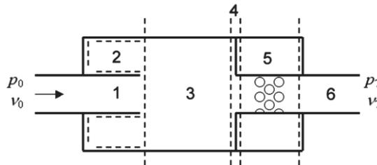
Figure 2 – Example of real muffler composed by several elements
