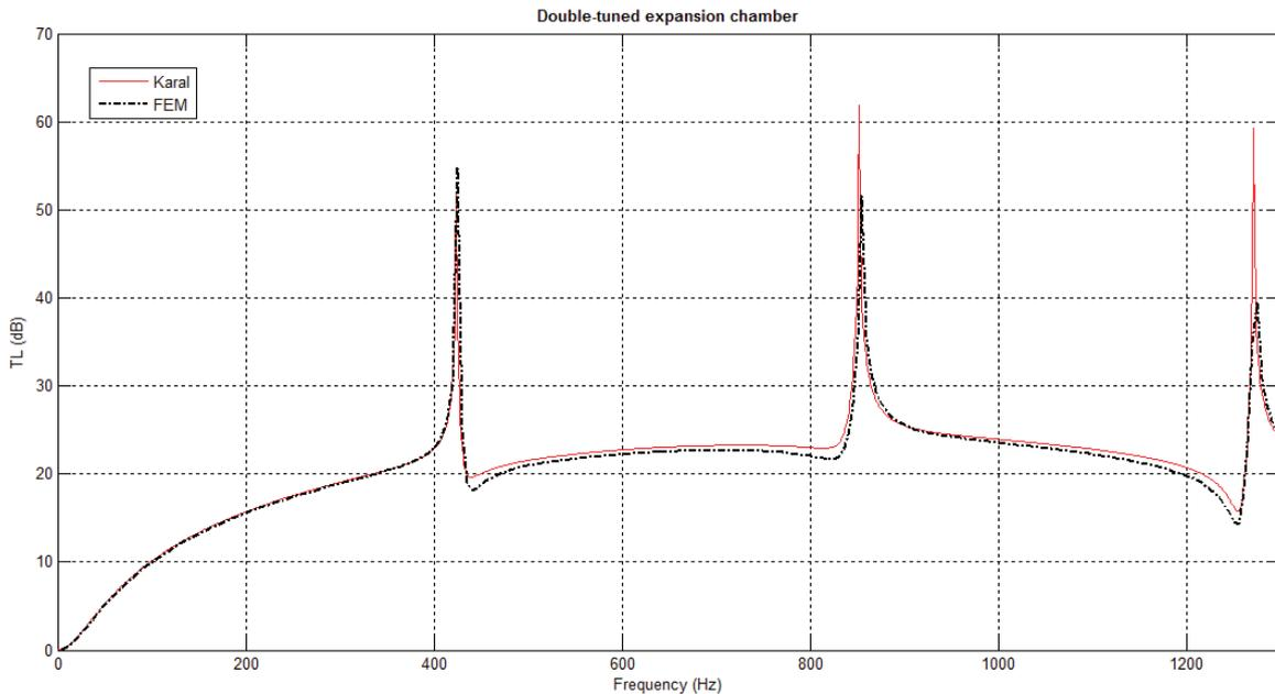
Figure 9 – Transmission loss comparison between 1D analytical model with Karal's end corrections factor and 3D FEM model for the double-tuned expansion chamber
