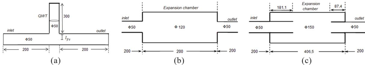
Figure 3 – Dimensions of the mufflers (a) quarter-wave-tube, (b) simple expansion chamber, (c) double-tuned expansion chamber
