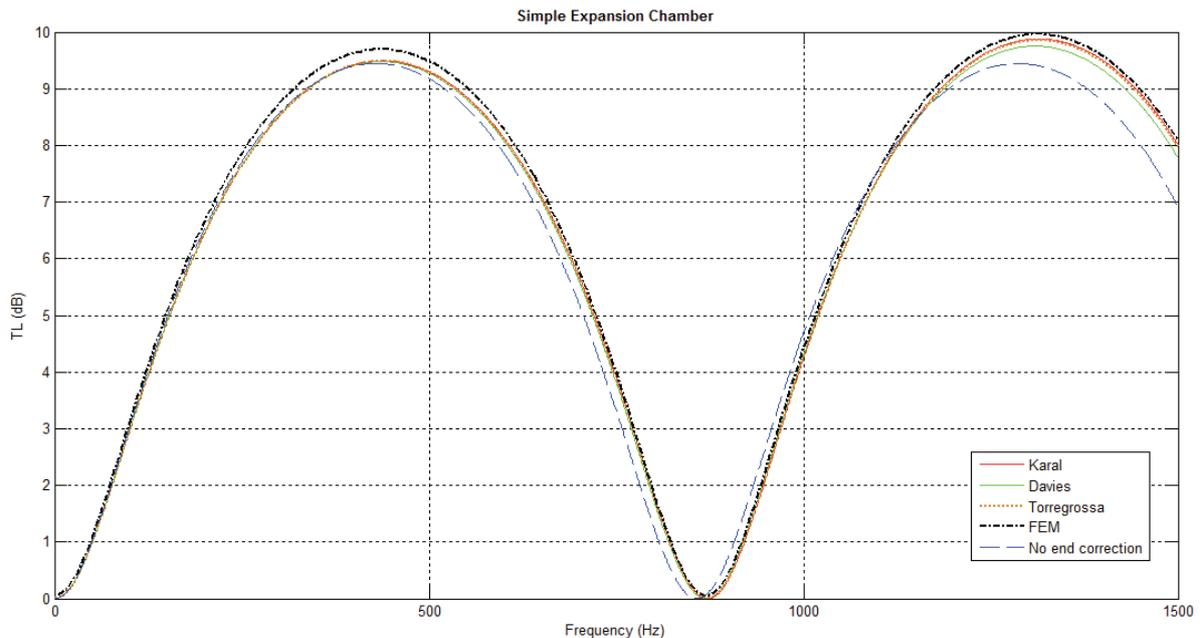
Figure 6 – Transmission loss comparison between 1D analytical model (with and without end corrections factor) and 3D FEM model for the simple expansion chamber
