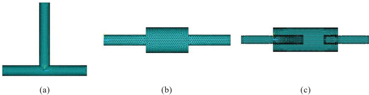
Figure 4 - Finite element mesh (a) quarter-wave-tube, (b) simple expansion chamber, (c) double-tuned expansion chamber
