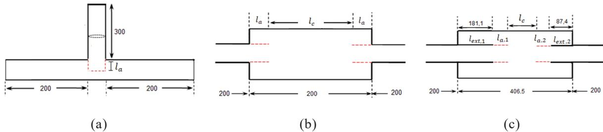
Figure 4 – Acoustic length correction (a) quarter-wave-tube, (b) simple expansion chamber, (c) double-tuned expansion chamber
