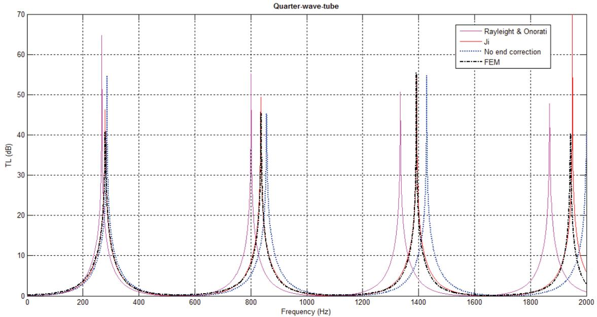
Figure 5 – Transmission loss comparison between 1D analytical model (with and without end corrections factor) and 3D FEM model for the quarter-wave-tube resonator
