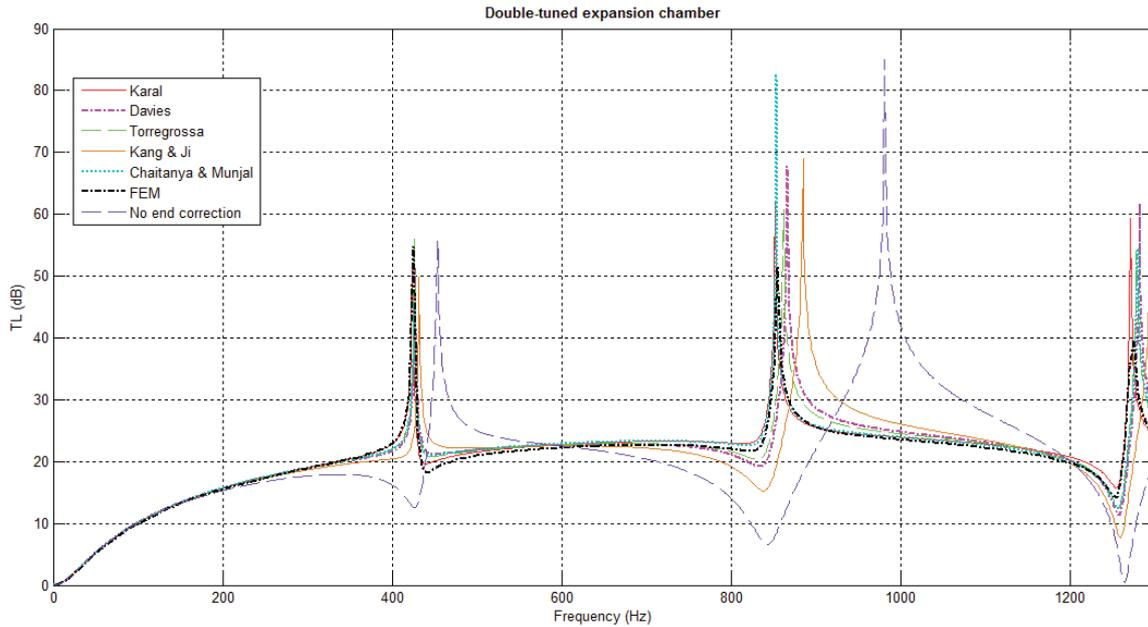
Figure 7 – Transmission loss comparison between 1D analytical model (with and without end corrections factor) and 3D FEM model for the double-tuned expansion chamber
