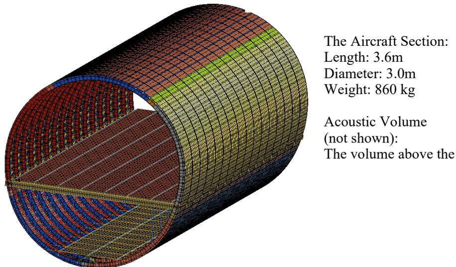
Figure 2 FE-Model of a schematic Turbo-Prop Aircraft structure.
