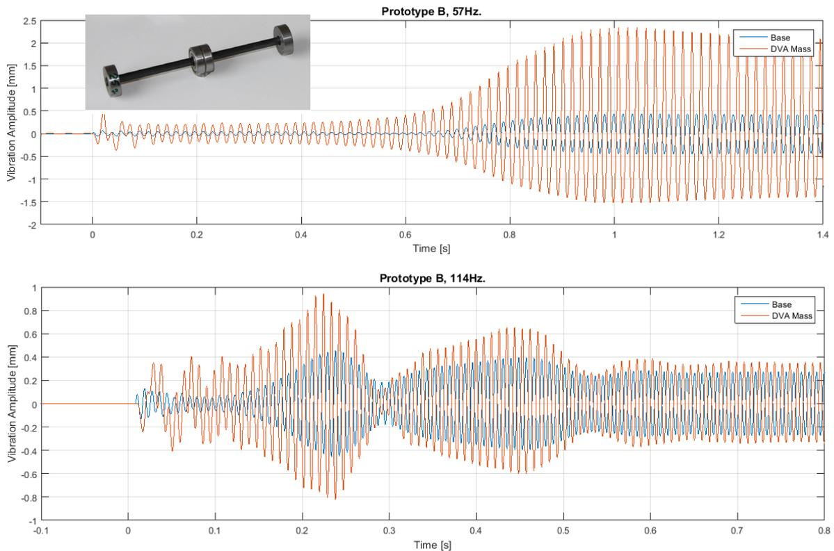
Figure 7 Prototype test results. The green curve show the vibration of the base (shaker) and the red curve is the vibration at one of the dynamic masses.
