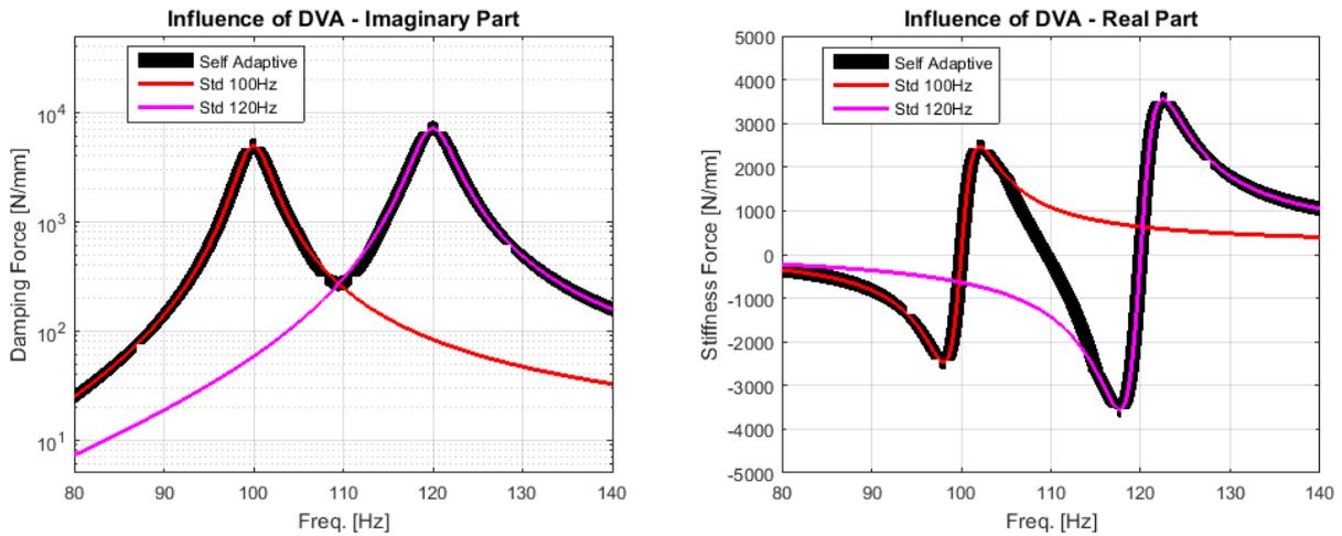
Figure 3 The dynamic force for the three different DVA types.
