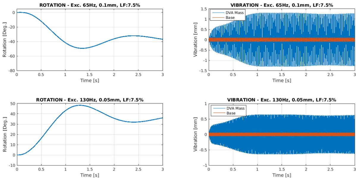
Figure 9 SA-DVA response for excitation at 65 Hz, 0.1mm [Peak], upper graphs, and for 130 Hz, 0.05mm [Peak], lower graphs.
