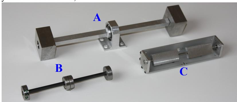
Figure 6 Self-Adaptive DVA prototypes. “A”: Large, “all-metal”, low damping version. “B”: Plastic/Fibre Glass elastic section. “C”: Prototype having different rotational inertia and circular elastic element.
