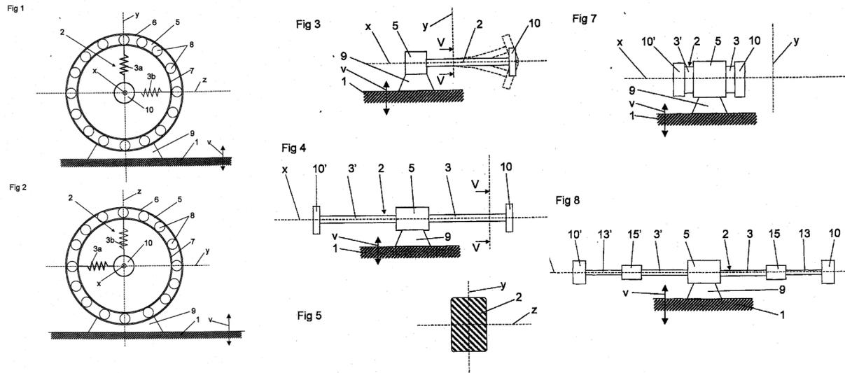
Figure 5 Design alternatives for Self-Adaptive Dynamic Vibration Absorber
