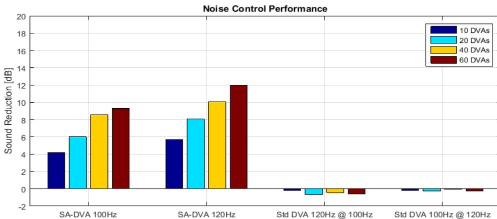
Figure 4 Noise control performance for DVA installation alternatives.
