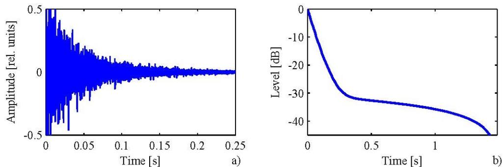
Figure 3 – Synthesized RIR with exponential decay and its backward integrated decay curve
