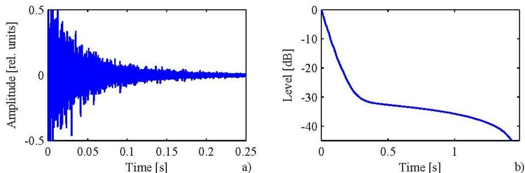
Figure 1 – RIR synthesized by the image source model (ISM) and its backward integrated decay curve
