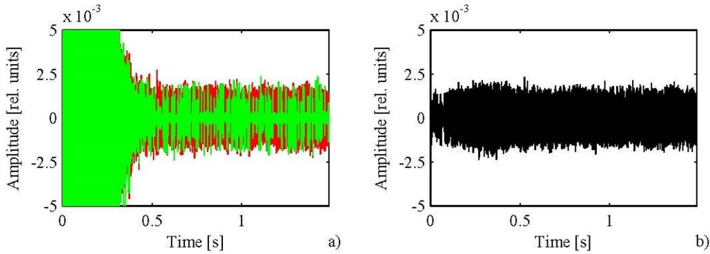
Figure 5 – RIR synthesized by the ISM with added -50 dB noise in the time domain a) before wavelet (without wavelet application) (---) and after wavelet (with Daubechies 2 wavelet at level 3) (—), as well as b) the difference of these RIRs
