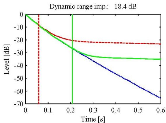
Figure 9 – IIDs of the RIR synthesized by the ISM: without the noise (···), with noise of level of -40 dB before the wavelet (---) and after applying the Daubechies 2 wavelet at level 6(—)
