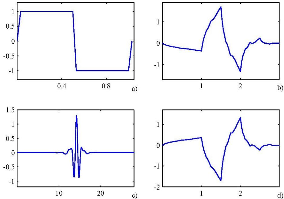
Figure 2 – Wavelet functions: a) Haar wavelet function, b) Deubechies wavelet function, c) Coiflet wavelet function and d) Symlet wavelet function
