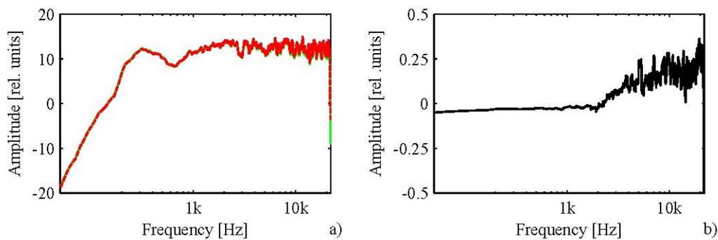
Figure 6 – RIR synthesized by the ISM with added -50 dB noise in the frequency domain a) before wavelet (without wavelet application) (---) and after wavelet (with Daubechies 2 wavelet at level 3) (—), as well as b) the difference of these RIRs
