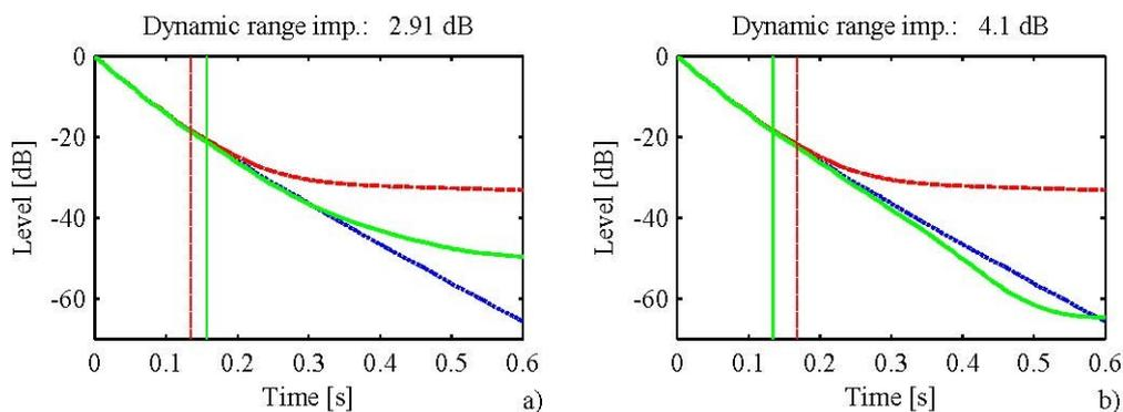
Figure 4 – IIDCs of noiseless RIR (reference curve  $\cdots$ ), noisy RIR before wavelet ( $---$ ) and after wavelet ( $-$ ), where the a) Daubechies 2 wavelet at level 3, and b) Daubechies 32 wavelet at level 8 are applied to the room response to the excitation (synthesized RIR generated by the ISM is used)
