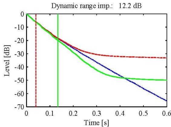
Figure 11 - IIDCs of the RIR synthesized by the ISM: without the noise ( $\cdots$ ), with noise of level of -50 dB before the wavelet ( $---$ ) and after applying the Daubechies 2 wavelet with *sqtwolog* for universal thresholding, *soft* thresholding and with level 3 ( $-$ )
