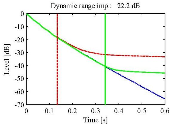
Figure 8 – IIDs of the RIR synthesized by the ISM: without the noise (···), with noise of level of -50 dB before the wavelet (---) and after applying the Haar wavelet at level 4 (—)
