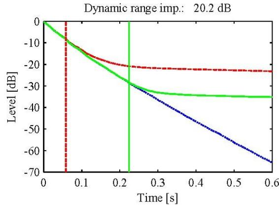
Figure 10 – IICs of the RIR synthesized by the ISM: without the noise (···), with noise of level of -40 dB before the wavelet (---) and after applying the Haar wavelet at level 6(—)
