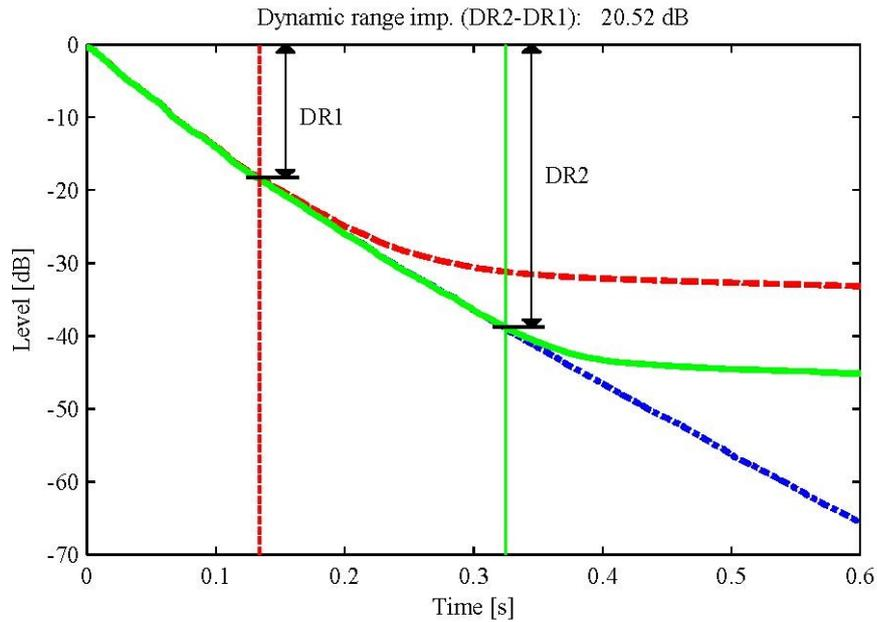
Figure 7 – IIDs of the RIR synthesized by the ISM: without noise - reference curve (···), with noise of level of -50 dB before the wavelet (---) and after applying the Daubechies 2 wavelet at level 3 (—)
