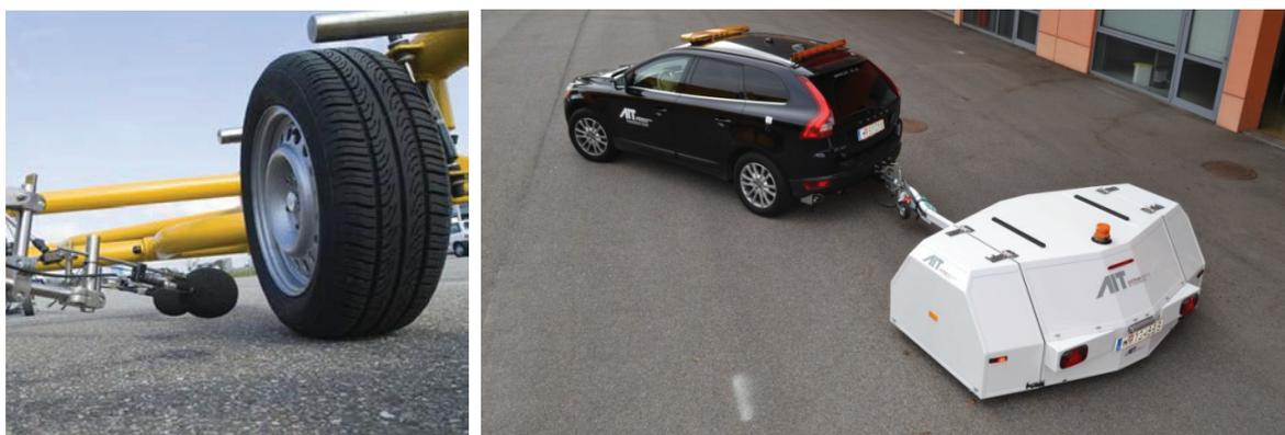
Figure 1: CPX trailer used for measuring road surface properties (left: the open trailer by DRD, right the closed trailer by AIT).
