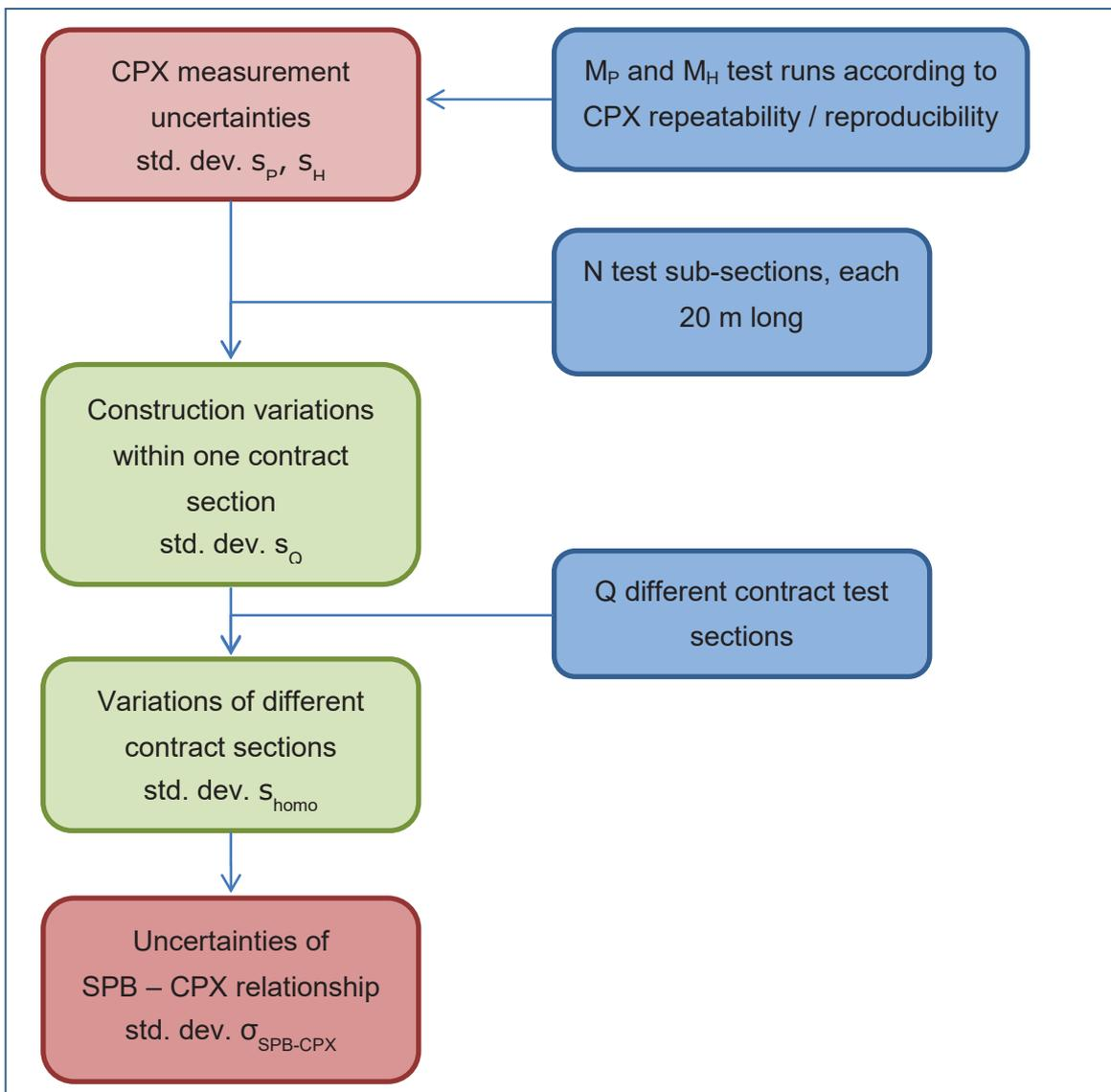
Figure 2: sources of uncertainty and variation for the characterization procedure including also a possible bridge to CNOSSOS-EU (3) (red: unwanted (measurement) uncertainties; green: acoustic variations of and within the road surface types, to be determined by the characterization method; blue: number of inputs for correct determination of uncertainties and variations).
