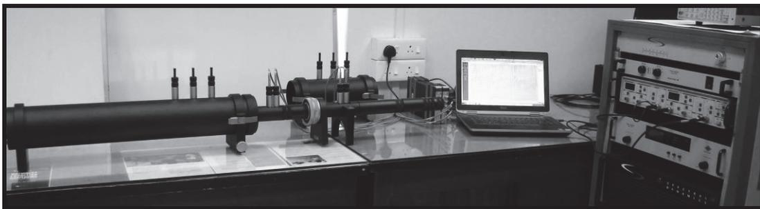
Figure 2-View of the impedance tube in the laboratory
