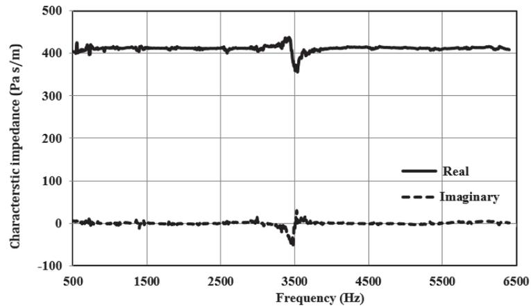
Figure 4-Measured characteristic impedance of air
