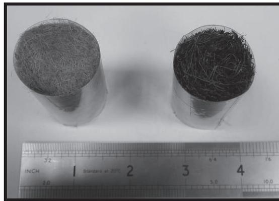
Figure 3-View of the natural fibrous samples (left-jute, right-coir)
