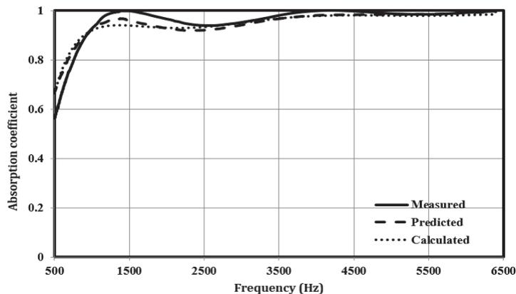
Figure 8-Sound absorbing coefficient for 50 mm sample length of jute felt.
