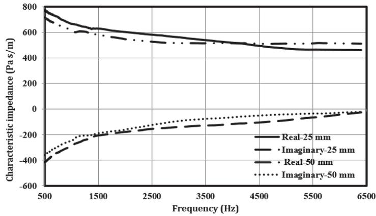
Figure 6-Measured characteristic impedance of jute felt sample of two different thicknesses
