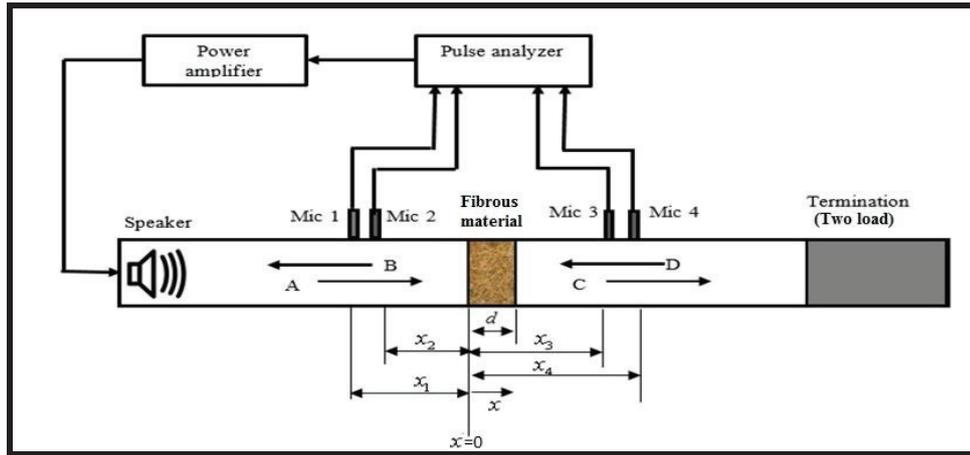
Figure 1–Schematic diagram showing the four microphone locations.
