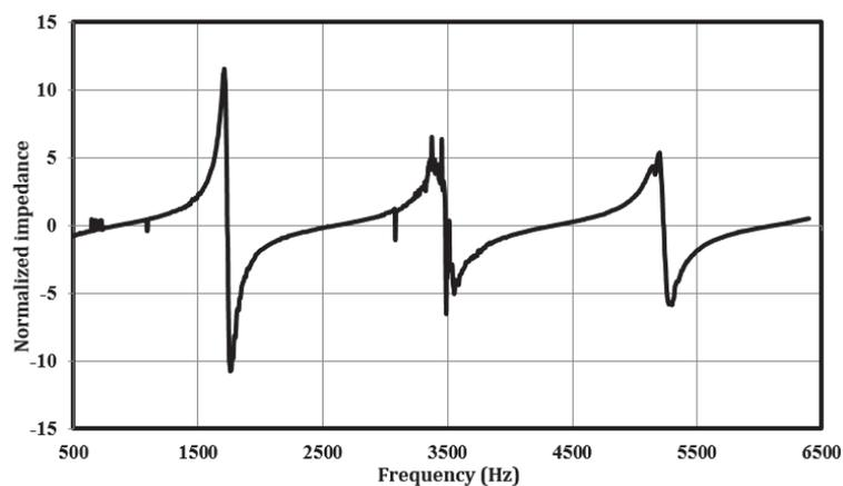
Figure 5-Estimated input impedance of a closed tube of 100mm length using the measured characteristic impedance of air
