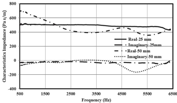
Figure 7-Measured characteristic impedance of coconut coir sample of two different thicknesses
