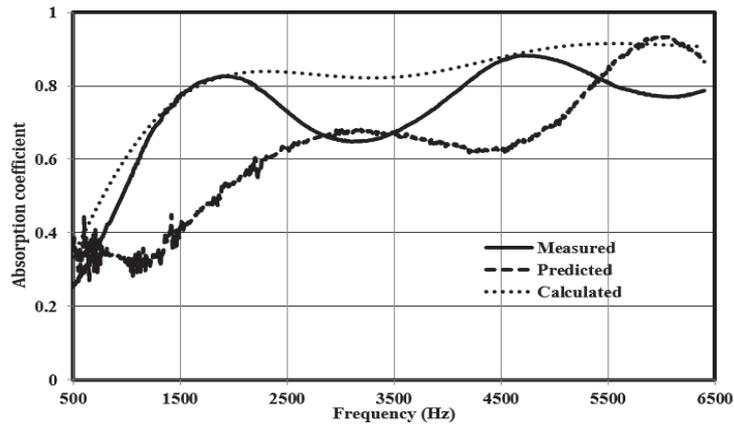
Figure 9-Sound absorbing coefficient for 50 mm sample length of coconut coir.
