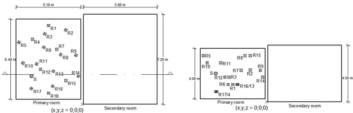
Figure 2 –Floor plan (left) and vertical cross-section (right) of the room system used in the computational model (without coupling) with source and receiver positions.
