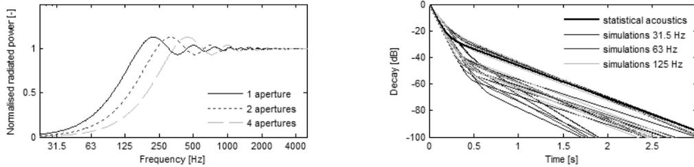
Figure 6 – Aperture transparency approximated as normalized radiated power of a piston in a plane boundary (left) and time domain simulation results compared to statistical acoustics results (right).
