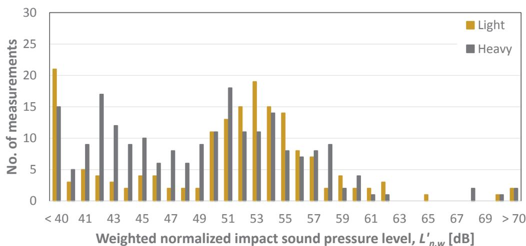
Figure 2 – Distribution of field measurements for impact sound pressure level,  $L'_{n,w}$ .
