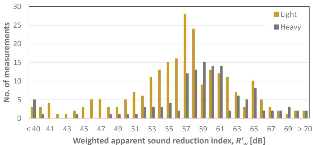
Figure 1 – Distribution of field measurements for sound reduction index,  $R'_w$ .
