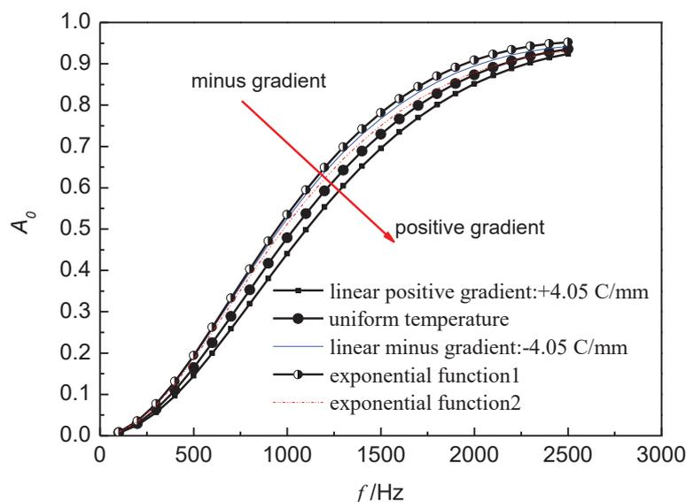
Figure 4 – Sound absorption coefficient of porous metals under different temperature field conditions [Ref.4]
