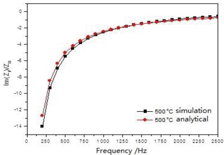
Figure 3 – Specific acoustic reactance of porous metal #1 at temperature of 500°C.
