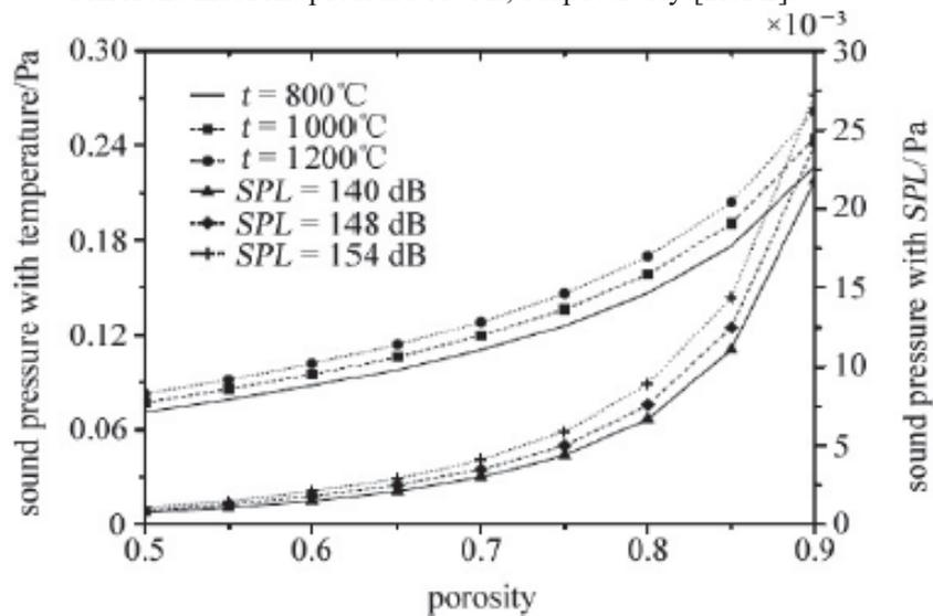
Figure 6 – Sound pressure for different values of porosity, at different temperatures, and at different incident pressure levels, respectively [Ref.2].
