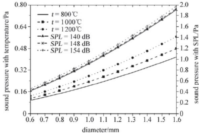
Figure 5 – Sound pressure for different values of wire diameter, at different temperatures, and at different incident pressure levels, respectively [Ref.2].
