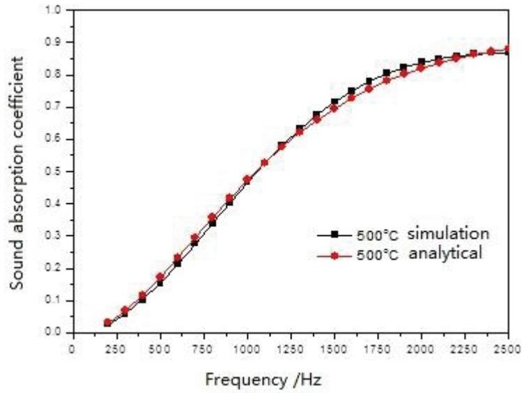
Figure 1 – Sound absorption coefficient of porous metal #1 at temperature of 500°C.
