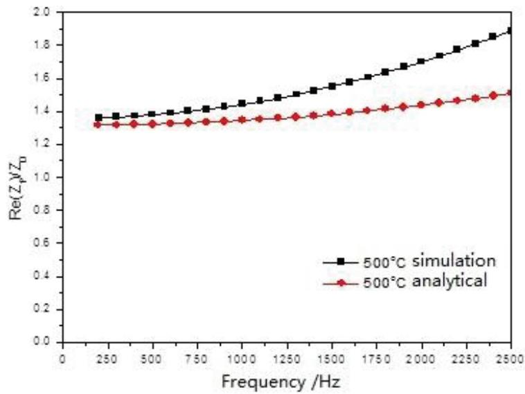
Figure 2 – Specific acoustic resistance of porous metal #1 at temperature of 500°C
